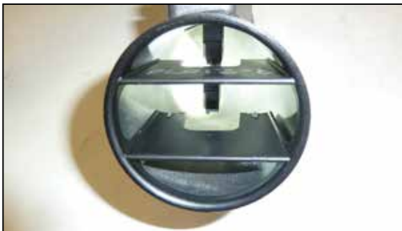
18. Apply small drops of the provided super glue to the lip of the mass air sensor grids and then install the grids into the K&N intake tubes as shown.
