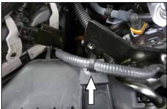
4. Unhook the mass air sensor wiring harness from the air filter housing.
