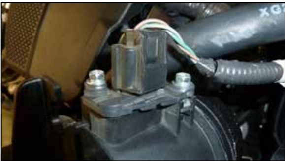
13. Disconnect the mass air sensor electrical connection from the driver side mass air sensor. Remove the driver side air filter housing assembly from the vehicle.
