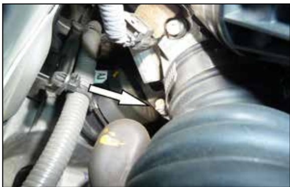
8. Loosen the clamp that secures the passenger side intake tube to the turbo and then separate the intake tube from the turbo.
