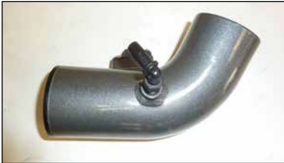
19. Install the provided 90 degree CCV fitting into the K&N passenger side intake tube as shown.
