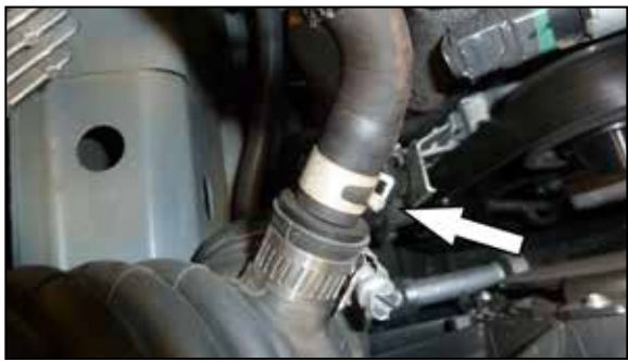
9. Release the Spring clamp that secures the CCV hose to the passenger side intake tube and then separate the hose from the tube, next remove the intake tube from the vehicle.
