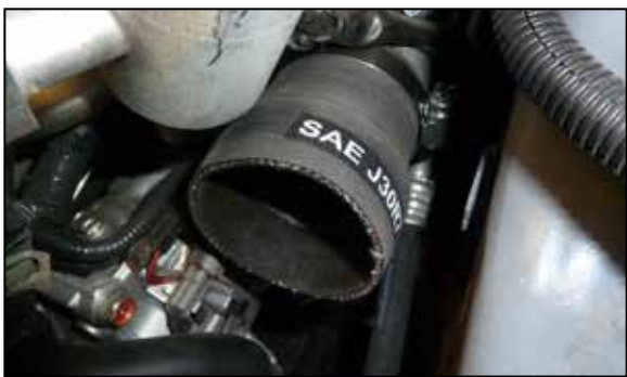
16. Install the step coupler provided onto the driver side turbo inlet and secure with the provided hose clamp.
