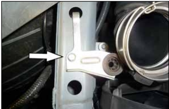
7. Remove the bolt that secures the lower air filter housing mount and then remove the mount from the vehicle.
