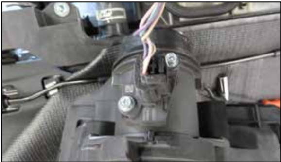
6. Disconnect the mass air sensor electrical connection from the passenger side mass air sensor. Remove the passenger side air filter housing assembly from the vehicle.
