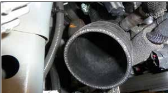
15. Install the elbow hose provided onto the passenger side turbo as shown. Do not secure the hose with the hose clamp yet as it will need to be adjusted for best fit in a later step.
