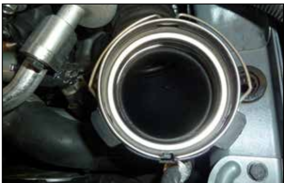
12. Release the locking clip that secures the factory air filter housing to the intake tube by pulling it away from the tube. NOTE: the picture is showing the clip in the released position while the air filter housing is removed.
