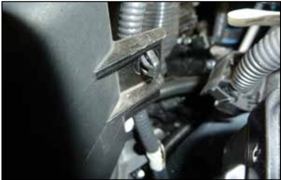
11. Unhook the mass air sensor wiring harness from the driver side air filter housing.
