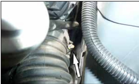
14. Loosen the hose clamp that secures the driver side intake tube to the turbo inlet and then remove the tube from the vehicle.
