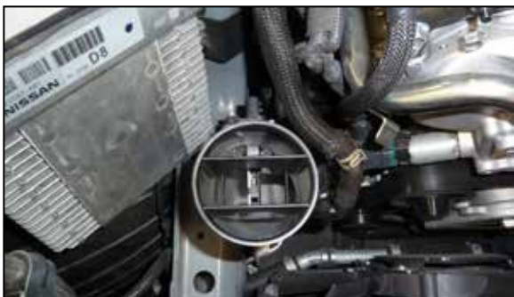
20. Install the passenger side K&N intake tube into the coupler but do not secure it with the hose clamp yet.
