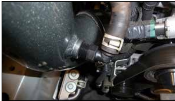
21. Connect the CCV hose to the 90 degree fitting installed into the K&N intake tube and secure with the factory spring clamp.
