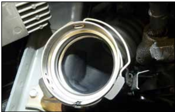
5. Release the locking clip that secures the factory air filter housing to the intake tube by pulling it away from the tube. NOTE: the picture is showing the clip in the released position while the air filter housing is removed.
