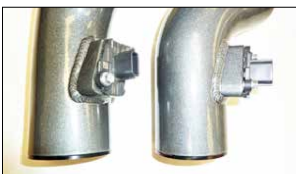
17. Remove the mass air sensors from the factory housings and install them into the K&N intake tubes as shown using the factory hardware.
