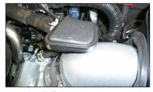
18. Install the PVC chamber into the grommet in the K&N® intake tube.
