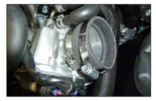
13. Install the provided coupler (08186) onto the throttle body and secure with the provided hose clamp.
