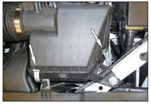
5. Release the two upper air filter housing retaining clips and then remove the upper air filter housing and intake boot from the vehicle.
