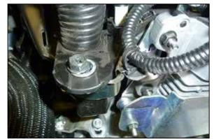
11. Remove the bolt that secures the wiring harness shown.
