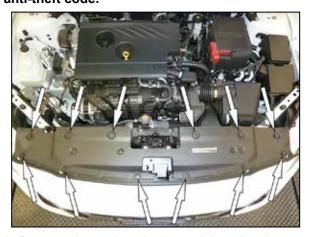
2. Remove the twelve plastic retaining clips that secure the upper valence and then remove the valence from the vehicle.
