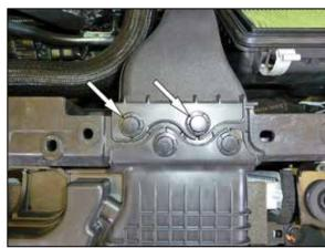
6. Remove the two plastic clips that retain the fresh air intake duct and then remove the duct from the vehicle.
