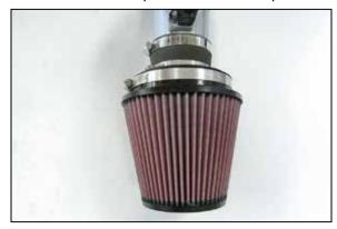
16. Install the K&N® air filter onto the filter adapter and secure with the provided hose clamp.
