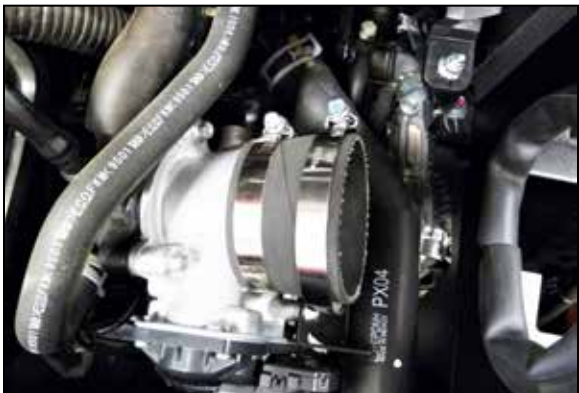
12. Install the provided coupler onto the throttle body and secure with the provided hose clamp.
