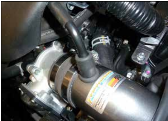
15. Install the factory ccv pipe into the grommet installed into the K&N intake tube.
