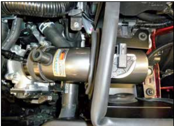
14. Install the K&N intake tube assembly through the heat shield and into the coupler at the throttle body, adjust the tube for best fit and then secure with the provided hose clamp.
