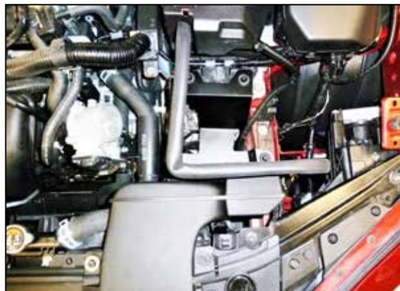
11. Install the heat shield assembly into the vehicle so the grommets engage the mounting studs. Secure the fresh air duct to the core support with the factory bolts.
