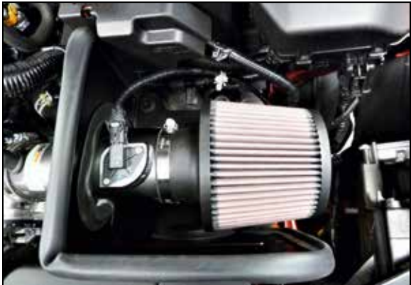
16. Install the K&N air filter onto the intake tube and secure with the provided hose clamp. Reconnect the maf sensor electrical connection.
