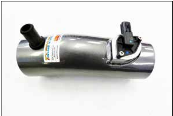
13. Remove the maf sensor from the factory air filter housing and then install it into the K&N intake tube. Install the provided ccv grommet into the intake tube and then install the provided TYPHOON decal.
