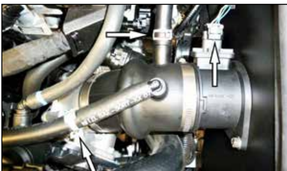
15. Reconnect the vent lines and secure with the factory spring clamps. Reconnect the mass air sensor electrical connection.
