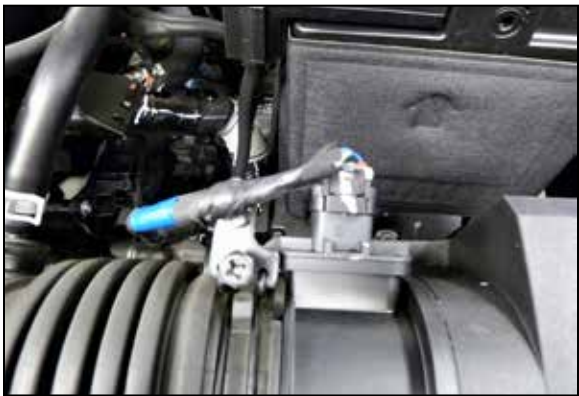
2. Disconnect the mass air sensor electrical connection.
