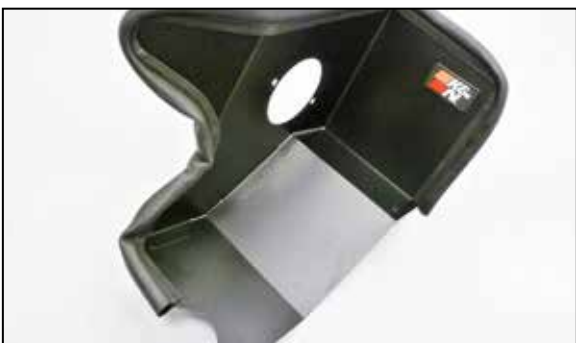
10. Install the edge trim around the heat shield as shown trimming off access. Install the K&N badge into the heat shield and secure with provided locking plate on the back side.
