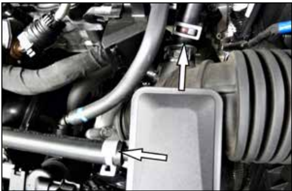
3. Release the two spring clamps that secure the vent hoses and then disconnect the vent hoses from the intake system.
