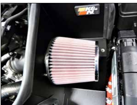
16. Install the K&N air filter onto the mass air sensor and secure with the provided hose clamp.
