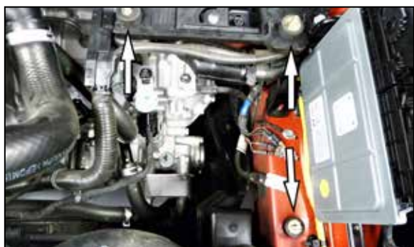
9. Install the three rubber mounted studs in the places shown.
