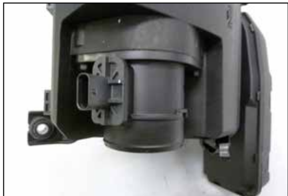
8. Remove the two bolts that secure the mass air sensor to the upper air filter housing and then remove the sensor from the housing.
