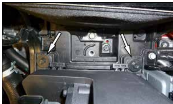
7. Remove the two rear air filter housing mounting bolts and then remove the complete intake assembly.
