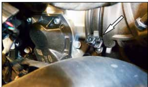
4. Loosen the hose clamp that secures the factory intake tube to the throttle body.
