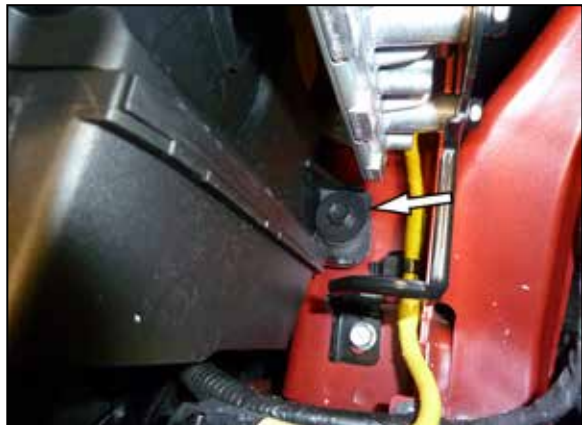
6. Remove the lower air filter housing retaining bolt.
