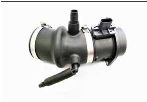
13. Install the factory mass air sensor into the K&N hose as shown but don't tighten the clamp.
