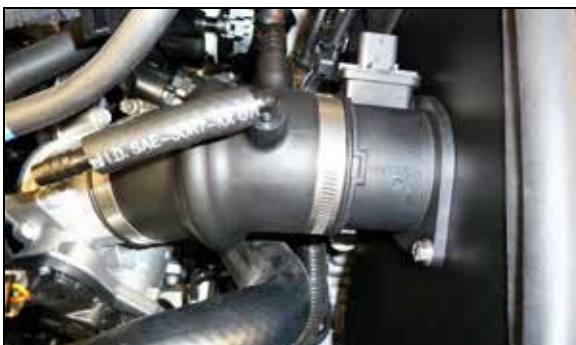
14. Install the hose/maf housing assembly onto the throttle body and into the heat shield. Adjust the maf housing so the holes line up and secure with the provided hardware. Adjust the hose for best fit and then secure with the provided hose clamps.
