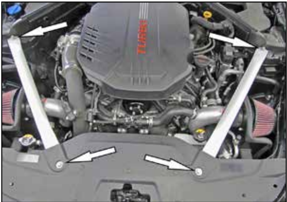
25. Reinstall both strut tower braces and secure with the factory hardware.
