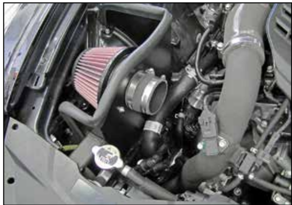
22. Install the coupling hose (084036) onto the filter adapter and secure with the provided hose clamp.
