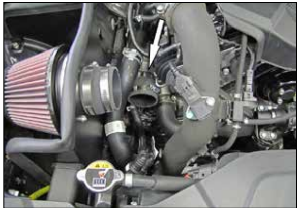
23. Install coupling hose (08638) onto the turbo inlet and secure with the provided hose clamp.
