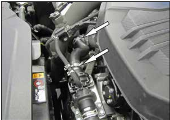
24. Install the passenger side intake tube (27678) into the coupler at the turbo and then into the coupler at the filter adapter, adjust the tube and heat shield assembly for best fit and then secure with the provided hose clamps. Install the driver side BOV hose onto the fitting on the K&N® intake tube and then onto the BOV valve. Secure with the factory spring clamps.
