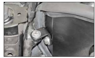
9. Install the provided "L" bracket (070066) onto the core support and heat shield as shown using the provided hardware, then tighten all of the heat shield mounting hardware.
