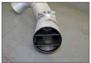
12. Install the air guide into the K&N® intake tube as shown.
