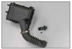
13. Remove the two screws securing the mass air sensor and then remove the mass air sensor from the air box.
