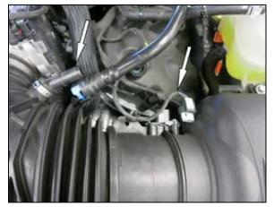
2. Release the locking tab and then disconnect the CCV hose quick connect fitting from the driver side intake tube. Release the locking clip and then disconnect the driver side MAF electrical connection.
