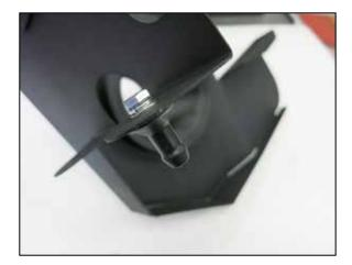
16. Install the remaining mounting stud to the passenger side heat shield using the provided hardware.
