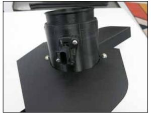
17. Remove the mass air sensor from the factory passenger side housing and then install it into the K&N passenger side housing using the provided hardware.
