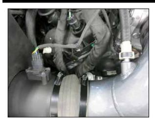
30. Connect the EVAP hose to the fitting on the K&N passenger intake tube. Reconnect the passenger side MAF electrical connection.
