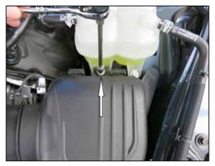
3. Remove the bolt that secures the driver side air filter housing to the inner fender.
