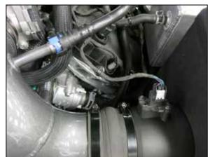
28. Connect the CCV to the fitting on the K&N driver side intake tube. Reconnect the MAF electrical connection.
