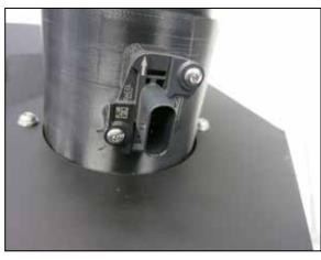
10. Remove the mass air sensor from the factory driver side maf housing and install it into the K&N driver side housing using the provided hardware.
