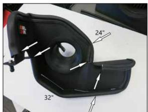
19. Install the edge trim onto the passenger side heat shield as shown. Install the K&N badge into the passenger side heat shield and secure with the provided locking tab.
