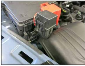
7. Pull back the relay from the fuse box assembly and set aside to allow clearance for air filter housing removal. **NOTE: K&N Engineering, Inc., recommends that customers do not discard factory air intake.**
