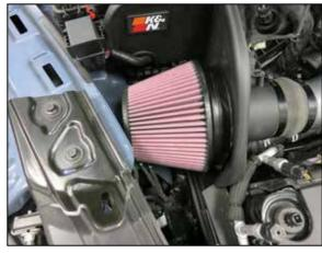
32. Install the passenger side K&N air filter and secure with the provided hose clamp.
