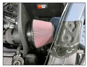
31. Install the driver side K&N air filter and secure with the provided hose clamp.
