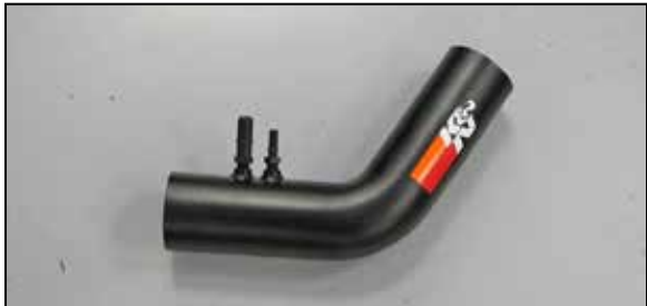
13. Install the provided quick disconnect fittings into the K&N® intake tube as shown. NOTE: NPT fittings are easy to cross thread. Install the vent fitting “hand” tight, then turn it two complete turns with a wrench.
