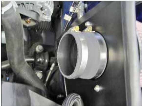
12. Install the provided coupler hose (08496) onto the filter adapter and secure with the provided hose clamp.
