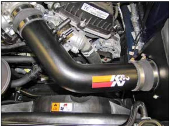
14. Install the K&N® intake tube into the coupling hoses and adjust for best fit, then secure the intake tube with the provided hose clamps.
