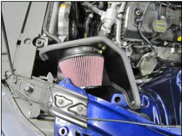
10. Install the K&N® air filter onto the adapter and secure with the provided hose clamp. Then secure the upper mounting bracket to the inner fender using the provided hardware.
