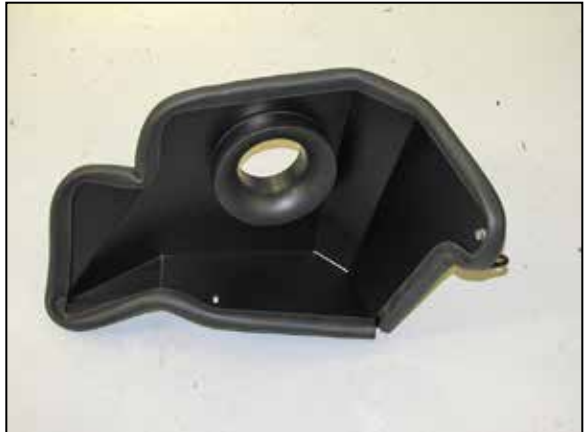
8. Install the edge trim onto the heat shield as shown. NOTE: Some trimming of the edge trim will be necessary.
