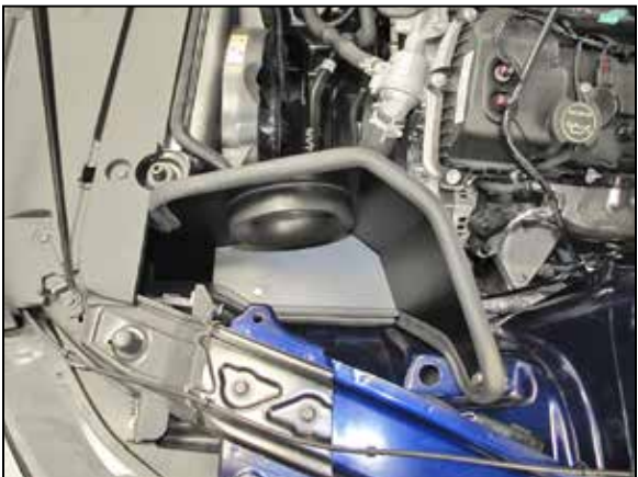
9. Install the heat shield onto the lower bracket installed in step #5 and secure with the provided hardware. Do not secure the upper bracket at this time.
