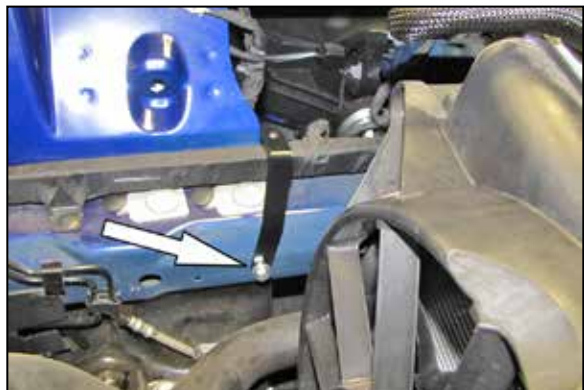
5. Install the lower heat shield bracket onto the fender using the provided hardware threaded into the existing threaded hole.
