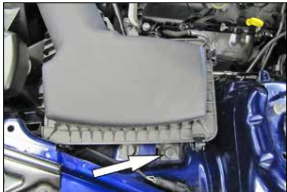
4. Remove the bolt which secures the air filter housing to the inner fender and then remove the air filter housing from the vehicle. NOTE: K&N Engineering, Inc., recommends that customers do not discard factory air intake.
