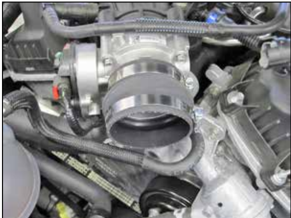
11. Install the provided hump coupler (5-323) onto the throttle body and secure with the provided hose clamp.
