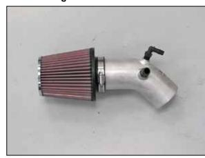
16. Install the K&N® air filter onto the K&N® intake tube and secure with the provided hose clamp.
