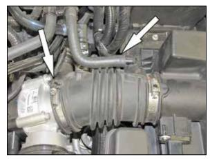
3. Disconnect the EVAP vent hose from the factory 90° fitting and then loosen the hose clamp securing the factory intake hose to the throttle body.
