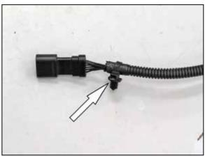
20. Install the provided "Mounting Tie Wrap" onto the female end of the mass air extension harness as shown.
