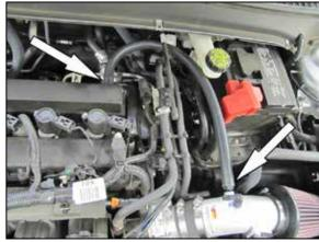
18. Install the provided crankcase vent hose onto the valve cover port and then onto the fitting installed into the K&N® intake tube as shown.
