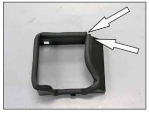
6. Install the provided top bulb edge trim onto the heat shield as shown.
