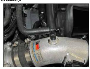
19. Connect the EVAP vent line to the 90° fitting installed into the K&N® intake tube as shown.
