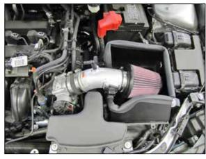
17. Install the Intake tube assembly into the silicone hose at the throttle body as shown, align for best fit and then secure with the provided hose clamp.
