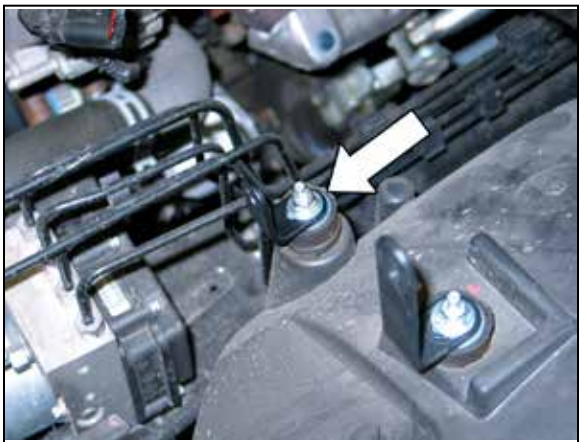
10. Install the provided heat shield mounting bracket (070066) onto the lower most rear factory air box mounting stud as shown.
