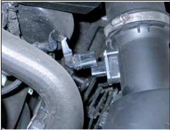
2. Disconnect the mass air sensor electrical connection.
