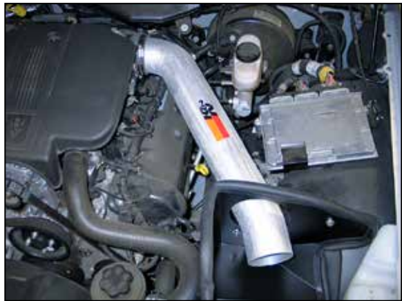
18. Install the intake tube into the heat shield and then into the silicone hose at the throttle body, secure the tube bracket to the heat shield with the provided hardware. Secure the intake tube to the silicone hose with the provided hose clamp.
