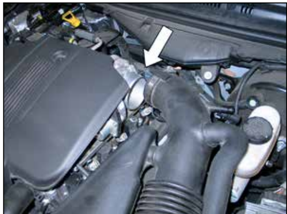
4. Loosen the hose clamp securing the factory intake tube to the throttle body and then disconnect the intake hose from the throttle body.
