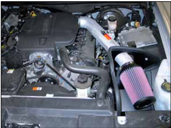
22. Reconnect the vehicle's negative battery cable. Double check to make sure everything is tight and properly positioned before starting the vehicle.
