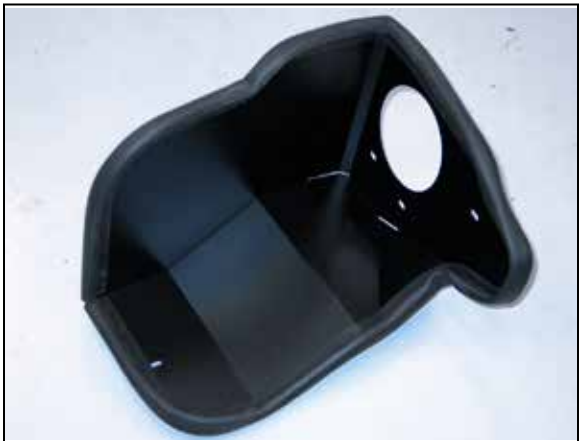
11. Install the provided edge trim onto the heat shield as shown. NOTE: Some trimming of the edge trim will be necessary.
