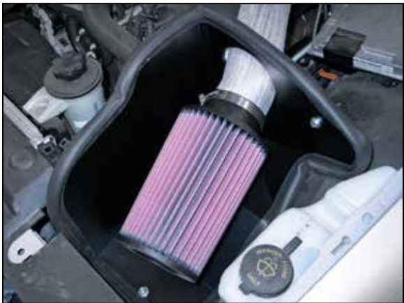
20. Install the K&N® air filter onto the intake tube and secure with the provided hose clamp. RC-5106DK is available to purchase separately. To learn more about Drycharger® filter wraps or look up color availability please visit http://www.knfilters.com ®.
