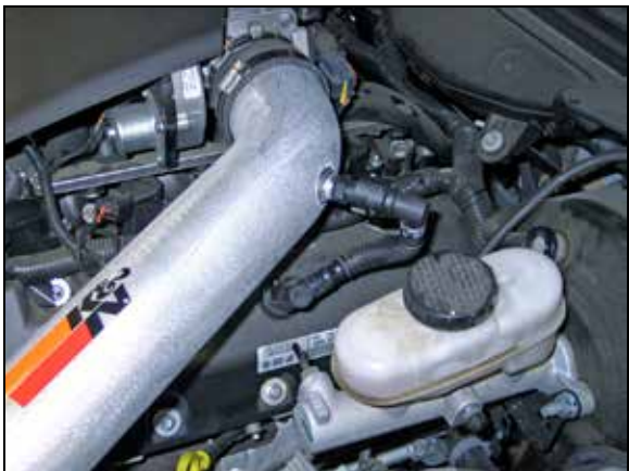
19. Connect the crank case vent hose to the fitting installed into the K&N® intake tube as shown.
