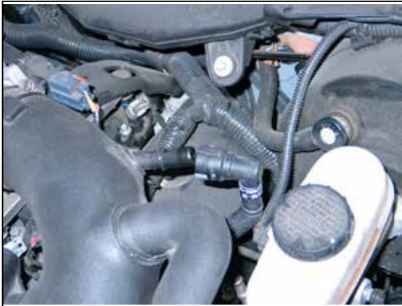
3. Disconnect the crank case vent hose from the intake tube.
