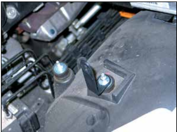
9. Install the provided heat shield mounting bracket (07195) onto the upper most rear factory air box mounting stud as shown.
