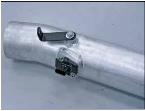
16. Install the tube mounting bracket (07805) onto the K&N intake tube as shown using the provided hardware.
