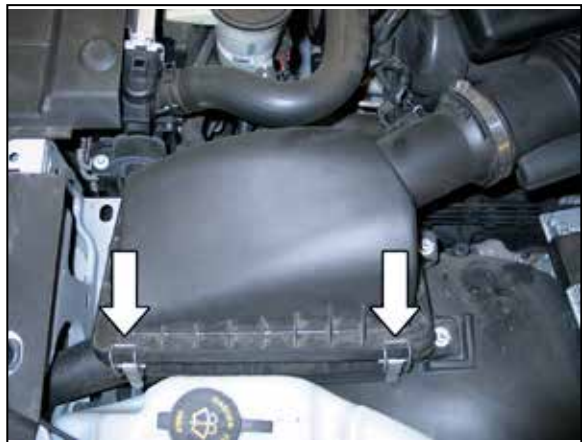
5. Release the two clips securing the upper air box to the lower air box.
