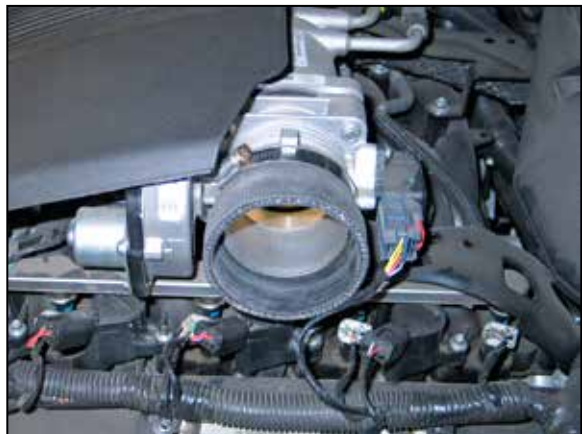
17. Install the provided silicone hose onto the throttle body as shown and secure with the provided hose clamp.
