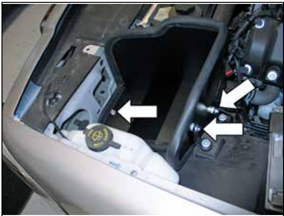
12. Install the heat shield assembly into the engine compartment and secure to the previously installed brackets and the forward factory air box mount with the provided hardware.
