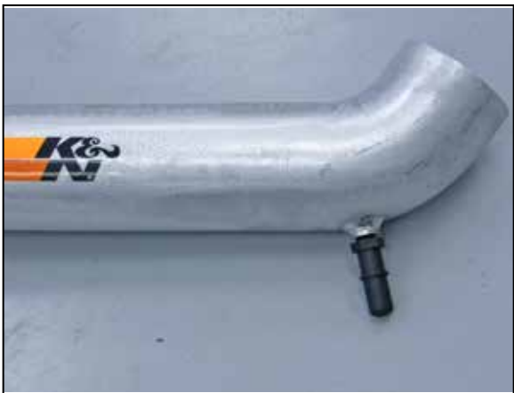
15. Install the provided crank case vent fitting into the K&N intake tube as shown. NOTE: NPT fittings are easy to cross thread. Install the vent fitting "hand" tight, then turn it two complete turns with a wrench.
