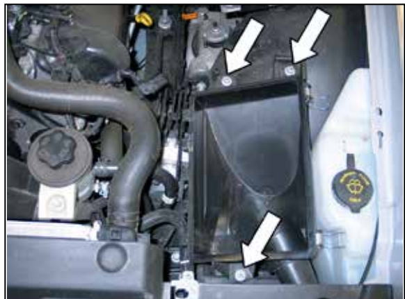
7. Remove the three nuts securing the lower air box into the engine compartment.
