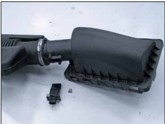
13. Remove the two screws securing the mass air sensor to the factory air box and then remove the sensor from the air box.
