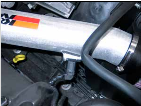
21. Reconnect the mass air sensor electrical connection.
