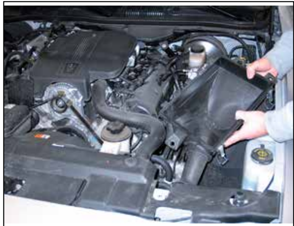
8. Remove the lower air box assembly from the vehicle. NOTE: K&N Engineering, Inc., recommends that customers do not discard factory air intake.
