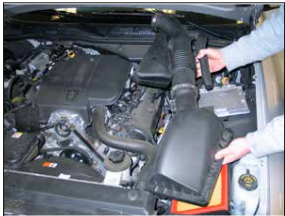
6. Remove the upper air box and intake tube assembly from the vehicle.
