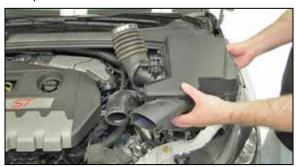
5. Remove the air box from the engine compartment.
