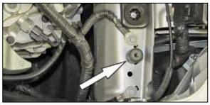
7. Install the provided rubber mounted stud into the inner fender as shown.
