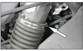
4. Loosen the hose clamp securing the intake hose to the plenum.
