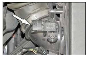
2. Disconnect the pressure sensor electrical connection.
