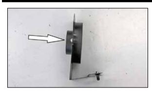
9. Install the filter adapter into the heat shield and secure with the provided hardware.
