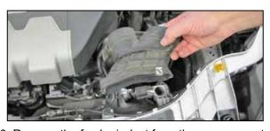
6. Remove the fresh air duct from the core support as shown.
