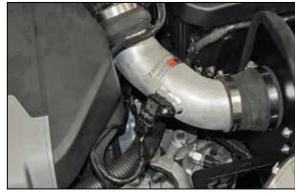
19. Reconnect the pressure sensor electrical connection.
