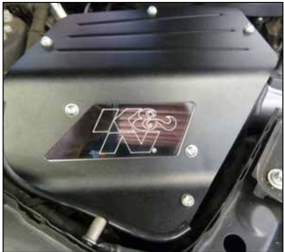
16. Install the lid onto the heat shield using the provided hardware.
