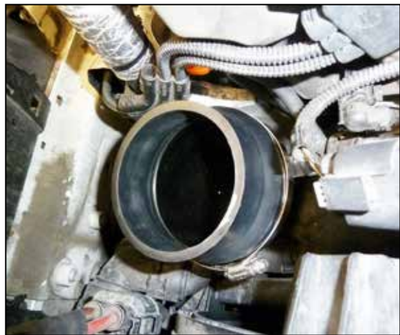
6. Install the provided coupler onto the turbo inlet and secure with the provided hose clamp.
