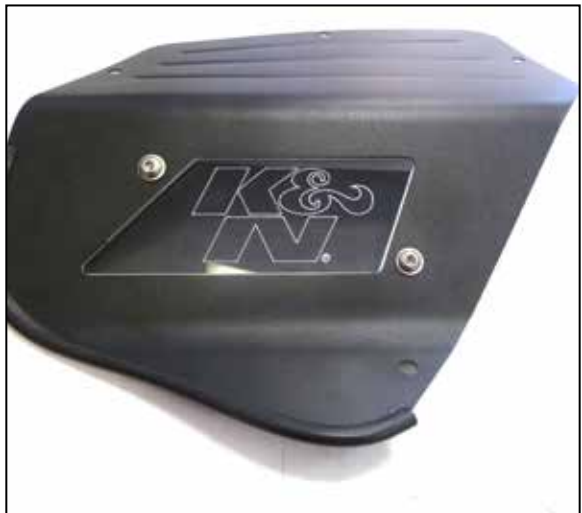
15. Install the provided edge trim onto the heat shield lid as shown using the provided super glue. Install the K&N window into the lid using the provided hardware and spacer.
