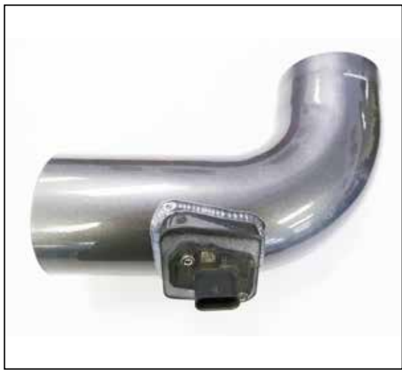
11. Remove the mass air sensor from the factory air filter housing and install it into the AEM intake tube using the provided hardware.
