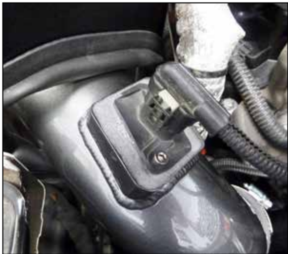
14. Connect the mass air sensor electrical connection.
