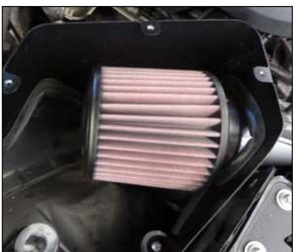
13. Install the air filter onto the intake tube and secure with the provided hose clamp. Adjust the tube and filter assembly for best fit and then secure the intake tube with the provided hose clamp.
