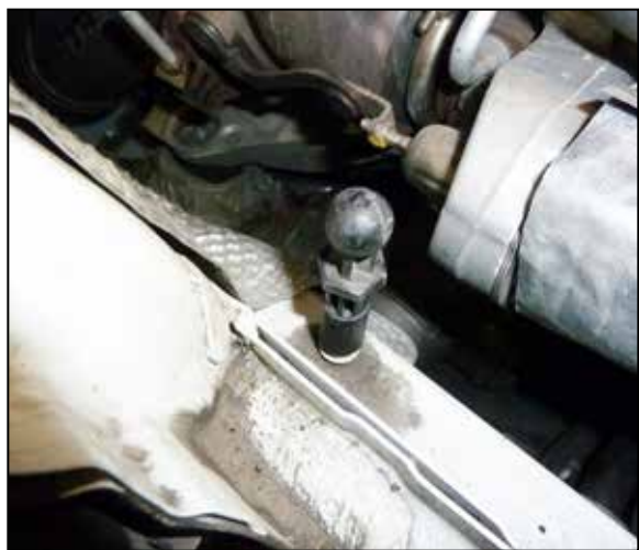
4. Remove the factory air filter housing mounting stud from the vehicle.
