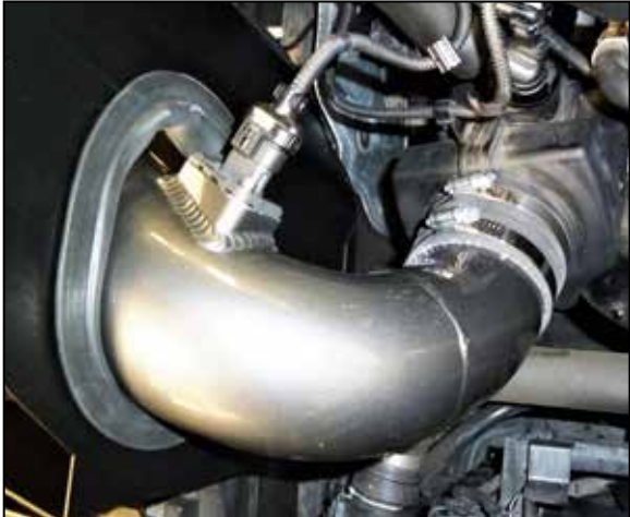
13. Install the intake tube through the hole in the heat shield and then into the coupler. Do not secure the hose clamp at this time. Connect the mass air sensor electrical connection.
