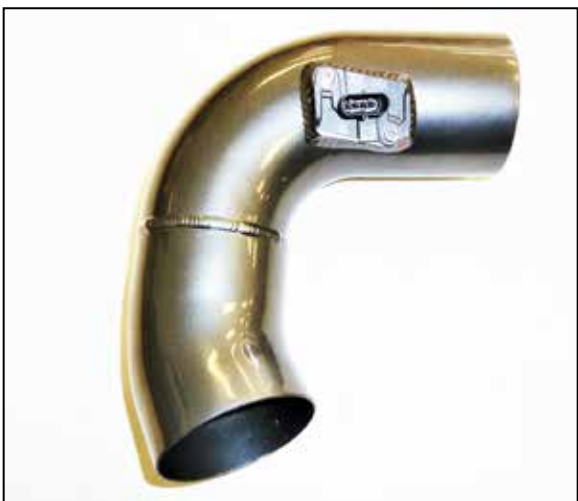
12. Remove the mass air sensor from the factory air filter housing and install it into the K&N intake tube and secure with the provided hardware.
