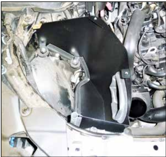
10. Install the heat shield into the vehicle so the mounting studs insert into the factory mounting grommets.
