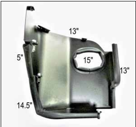
9. Install the edge trim onto the heat shield as shown.
