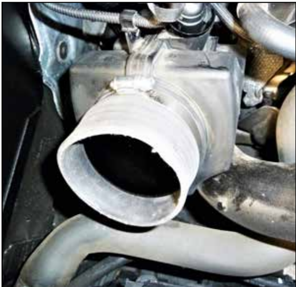
11. Install the provided coupler onto the plenum and secure with the provided hose clamp.
