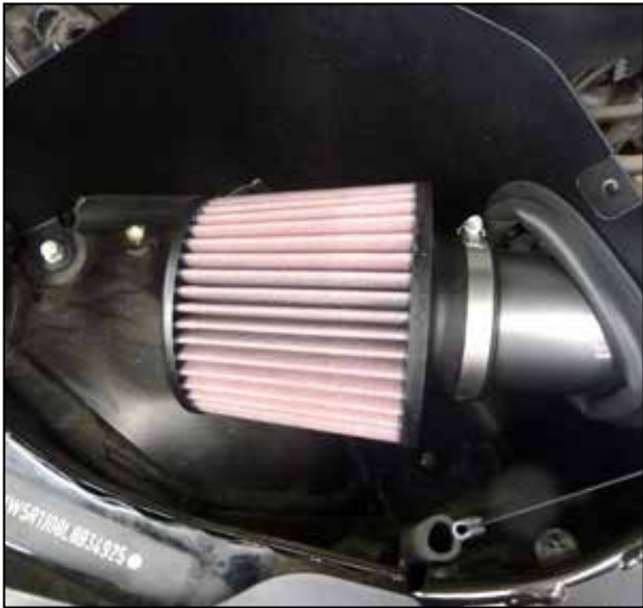
14. Install the air filter onto the intake tube and secure with the provided hose clamp. Adjust the tube for best fit and then secure the hose clamp.
