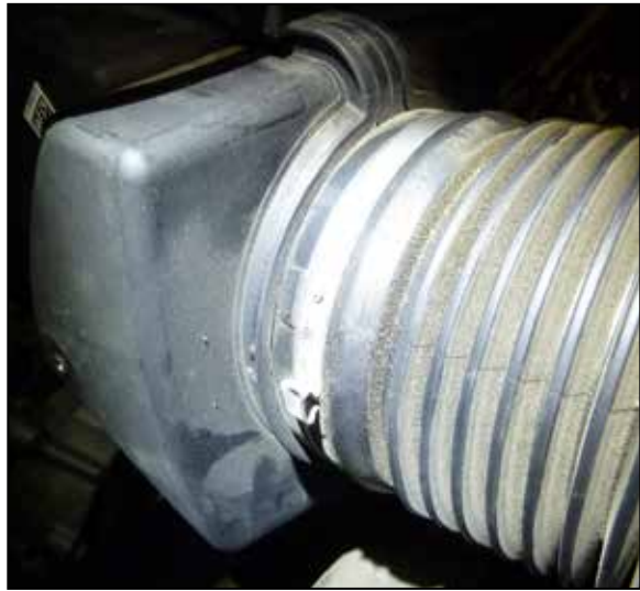
6. Cut the one-time use clamp that secures the intake hose to the intake plenum and then remove the intake tube from the vehicle.
