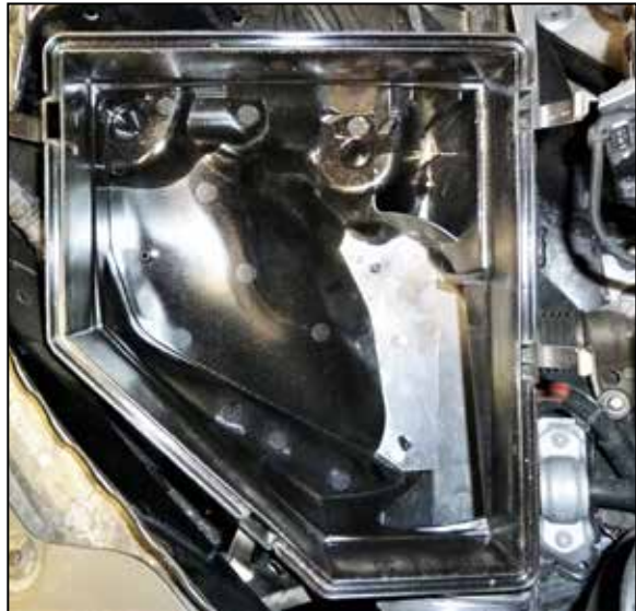
5. Pull the lower half of the air filter housing straight up and remove it from the vehicle.
