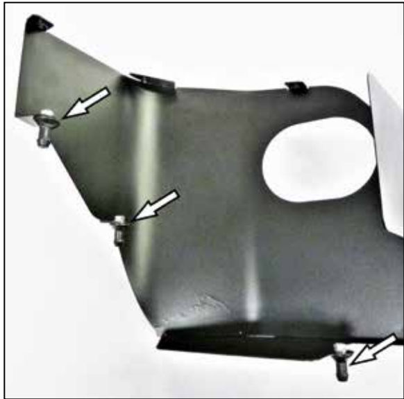
7. Install the three mounting studs provided onto the heat shield as shown.
