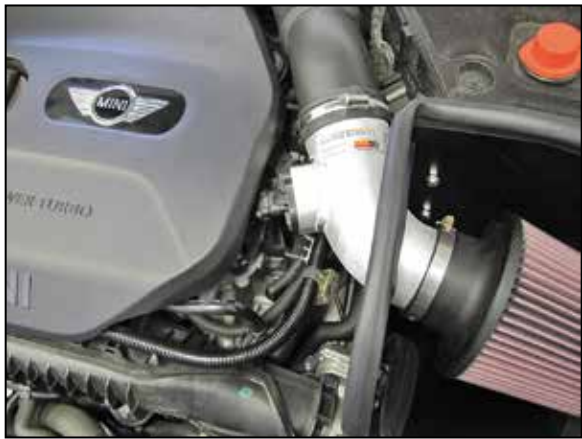
17. Reconnect the mass air sensor electrical connection.
