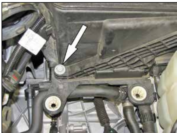
11. Remove the battery cover bolt shown. NOTE: This bolt will be reused in the next step.
