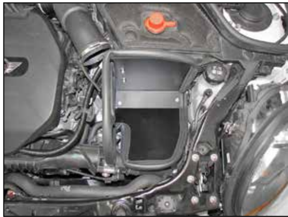
12. Install the heat shield into the vehicle so the mounting studs engage the mounting grommets and then secure the heat shield with the battery cover bolt removed in the previous step.
