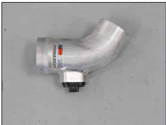
14. Install the mass air sensor into the K&N® intake tube and secure with the provided hardware.
