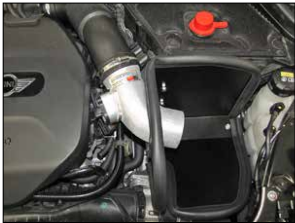
15. Install the K&N® intake tube into the heat shield and turbo inlet hose and then secure the tube with the provided hose clamp.
