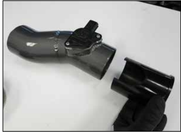
13. Remove the mass air sensor from the factory housing and install it into the K&N intake tube and secure with the factory screws.
