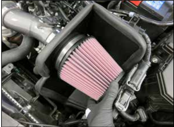
18. Install the K&N air filter onto the filter adapter and secure with the provided hose clamp.
