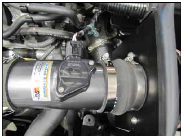
16. Reconnect the mass air sensor electrical connection.
