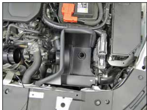
10. Install the heat shield and secure with the provided hardware.
