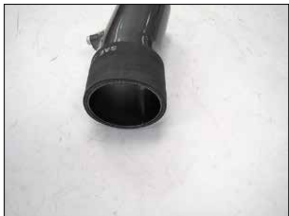
12. Install the provided coupling hose (08711) onto the intake tube so that it slides all the way on. Do not secure the hose now.
