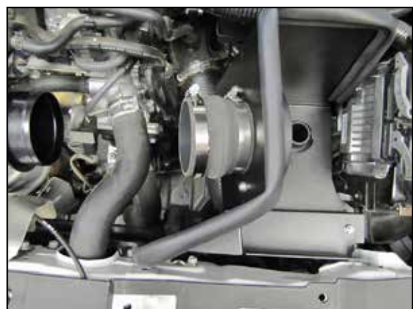
11. Install the provided coupling hose (087121) onto the filter adapter and secure with the provided hose clamp.
