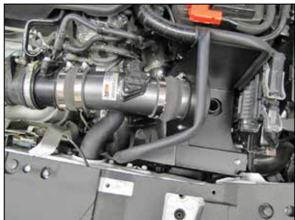
14. Install the K&N® intake tube into the coupler at the filter adapter and align with the turbo inlet pipe, slide the coupler back onto the turbo inlet pipe and adjust the tube for best fit. Secure the intake tube with the provided hose clamps.
