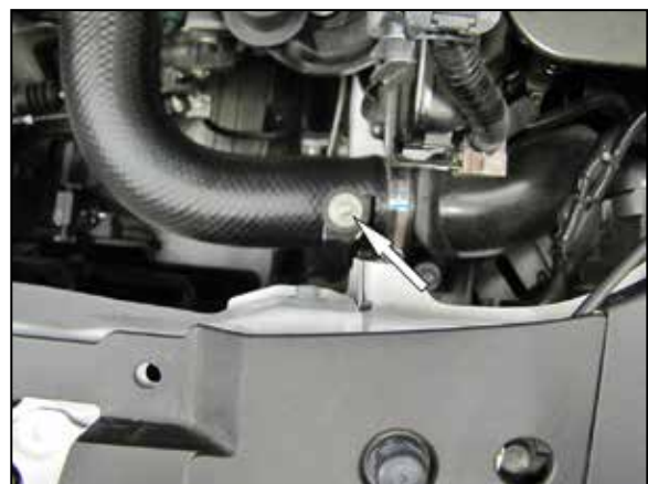
9. Install the provided rubber mounted stud onto the factory air filter housing mounting location.
