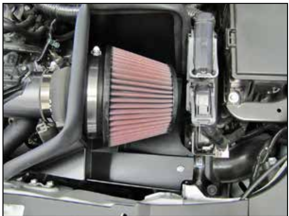
15. Install the K&N® air filter onto the filter adapter and secure with the provided hose clamp.
