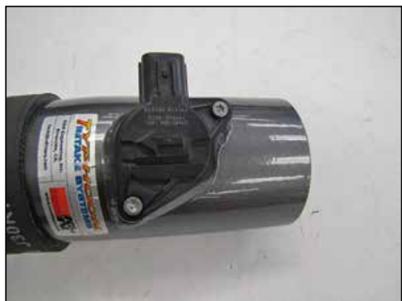
13. Remove the mass air sensor from the factory air filter housing and then install it into the K&N® intake tube and secure with the provided hardware.
