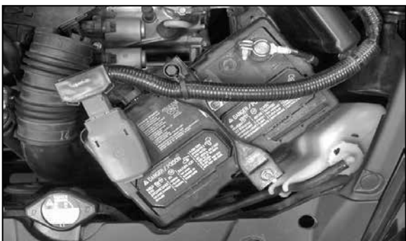
21. Loosen the positive battery cable and unclip the battery wire harness, adjust battery cable as shown. Then resecure the battery.
