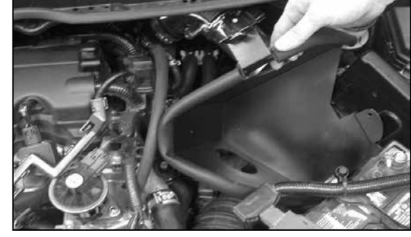
23. Slide the provided hose clamp onto the K&N intake tube, then install the heat shield. NOTE: On automatic transmission equipped vehicles, it will be necessary to remove the air filter and heat shield from the vehicle to check the transmission fluid level.
