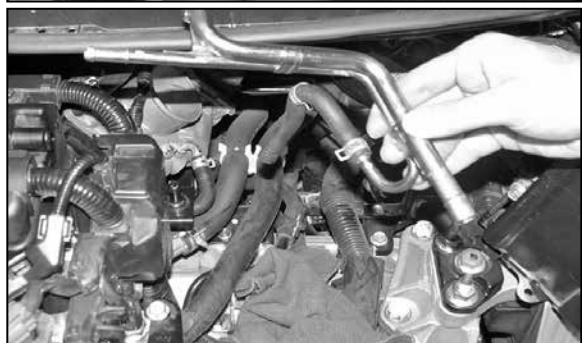
11. Using pliers, remove the coolant hose from the thermostat housing and the throttle body adaptor (a small amount of coolant may drain, have a cup ready to catch the fluid).
