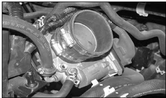
13. Install the silicone hose and hose clamps onto the throttle body as shown.
