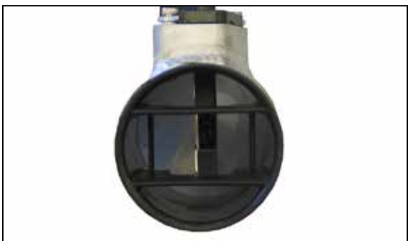
15a. Install the provided venturi into the end of the intake tube as shown. NOTE: Apply a thin coat of the provided super glue to the lip of the venturi.
