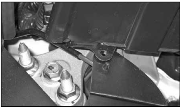
24. Install clip to the hydraulic line then attach to hole in heat shield.
