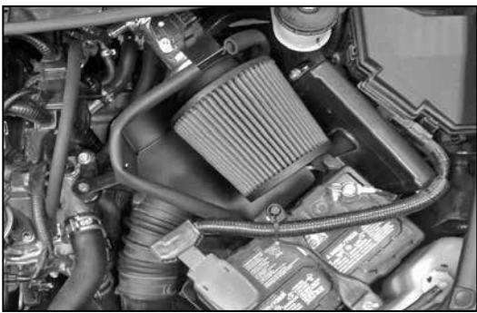
26. Install the air filter onto the K&N® intake tube.
