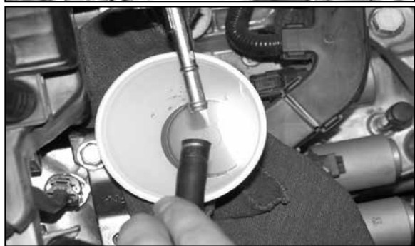
15a. Install the provided venturi into the end of the intake tube as shown. NOTE: Apply a thin coat of the provided super glue to the lip of the venturi.
