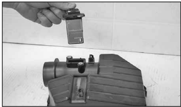
14. Loosen and remove the two screws that hold the MAF sensor to the factory airbox and remove the MAF sensor.
