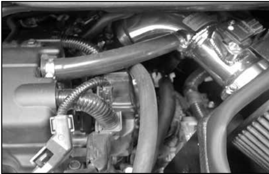
27. Attach the provided CCV-hose with #8 hose clamps, from the engine valve cover to the K&N® intake tube as shown.
