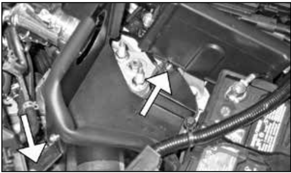
25. Attach the "L" bracket to the heat shield, and then install a bolt through the the hole on the ECU bracket to the threaded boss on the heat shield. Then attach the factory air inlet hose to the heat shield.
