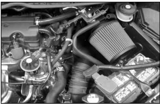
33. Reconnect the vehicle's negative battery cable. Double check to make sure everything is tight and properly positioned before starting the vehicle.
