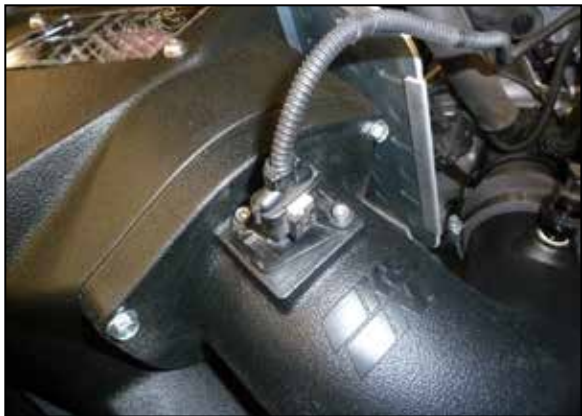
16. Reconnect the temp sensor electrical connection.
