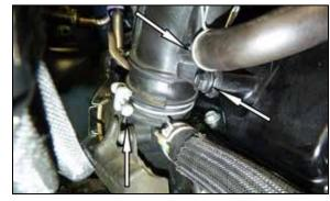
5. Disconnect the PCV hose from the passenger side lower intake tube, Remove the intake tube mounting bolt then loosen the hose clamp securing the intake tube to the turbo inlet and remove the tube from the vehicle.
