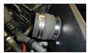
13. Install the provided hump couplers onto the filter adapters and secure with the provided hose clamps.
