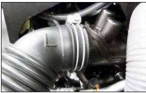
4. Loosen the hose clamps that secure the factory upper intake tubes and then remove the upper housings and intake tubes. NOTE: K&N Engineering, Inc., recommends that customers do not discard factory air intake.
