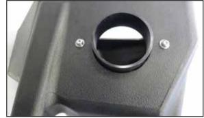
10. Install the filter adapters into the K&N air filter housings and secure with the provided hardware.
