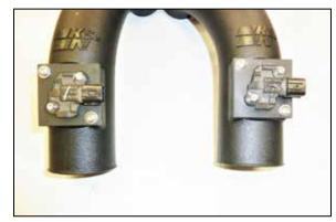
15. Using the provided adapter plates and gaskets, install the mass air sensors into the K&N intake tubes as shown.
