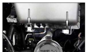
3. Release the retaining clips that secure the upper air filter housings.
