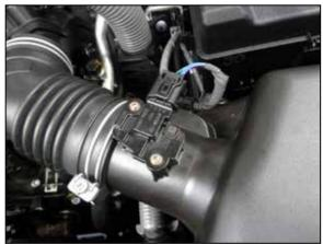
2. Disconnect the passenger and driver side mass air sensor electrical connection and unhook the harness's mounting clips.
