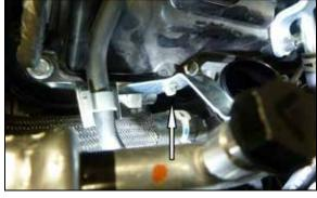
7. Remove the bolt that secures the driver side intake tube mounting bracket and then remove the bracket from the vehicle.
