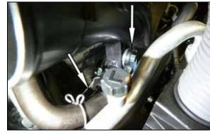
6. Disconnect the PCV hose from the driver side lower intake tube, Remove the intake tube mounting bolt then loosen the hose clamp securing the intake tube to the turbo inlet and remove the tube from the vehicle.
