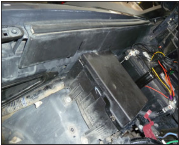
25. Re-install the under-hood plastic fender liner.
