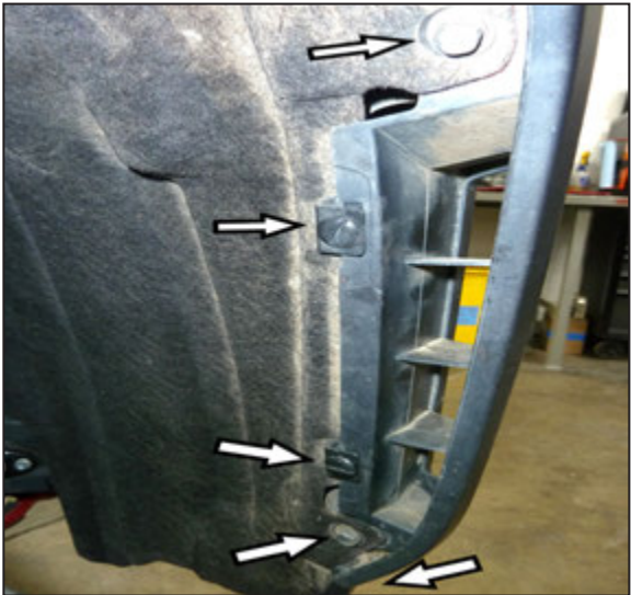
3. Remove the three bolts and two plastic retaining clips that secure the inner fender apron to the front bumper fascia.
