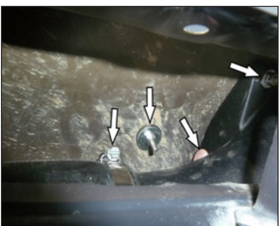
24. Install the rubber washers, large fender washers and nuts onto the studs. Tighten all the hardware evenly to secure the snorkel to the fender and the inner tube to the snorkel. Check the alignment of the fresh air duct and then tighten the hose clamp to secure it to the snorkel tube.
