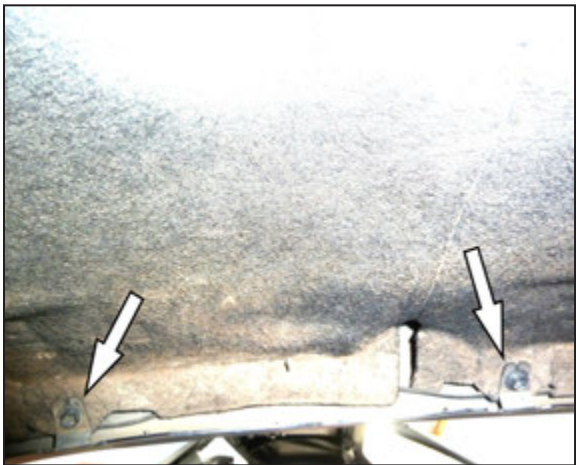
4. Remove the two bolts that secure the inner fender apron to the fender.
