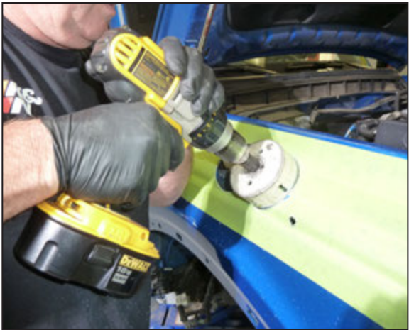
14. Drill the two air duct holes with a 3-3/4" hole saw.
