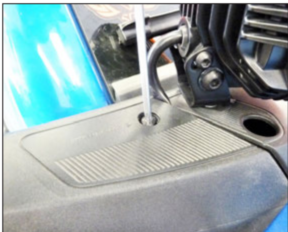
20. Remove the factory bolt show from Cowl/rear view mirror.
