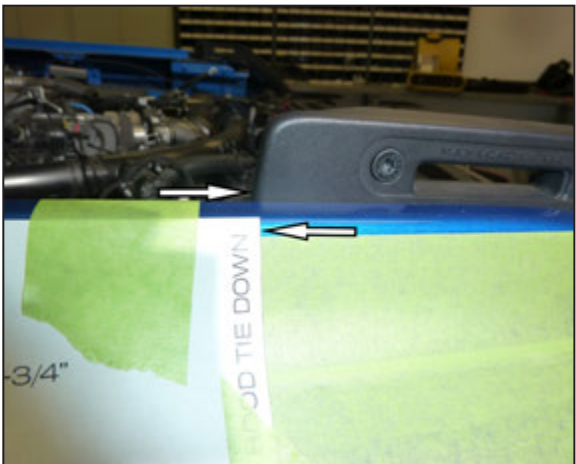
11c. The front edge of the pattern should align with the back edge of the fender sight.
