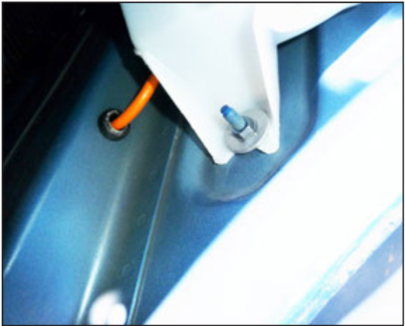
8. Remove the nut and push pin that secures the washer fluid tank and then remove the tank. Use caution to avoid damaging the tank or hoses, maneuver the tank back and forth for it to drop down from the fender.
