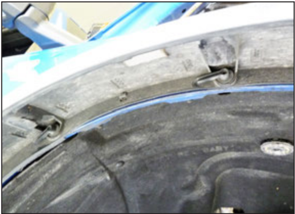
3. On vehicles equipped with extended fender flares, rotate the quarter turn fasteners counterclockwise to release and then remove the flare from the vehicle.
