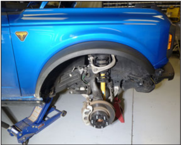
2. Jack up the front passenger side of the vehicle and support with a jack stand. Remove the front tire.
