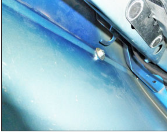
23. Install the two 8mm bolts with the fender washer. Do not tighten.
