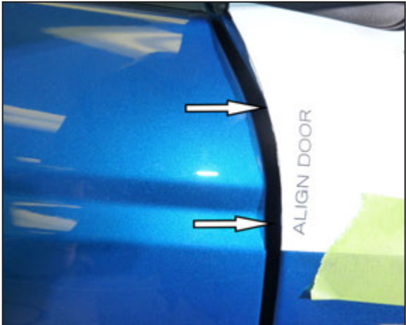
11b. The rear edge of the pattern should align with the edge of the fender.
