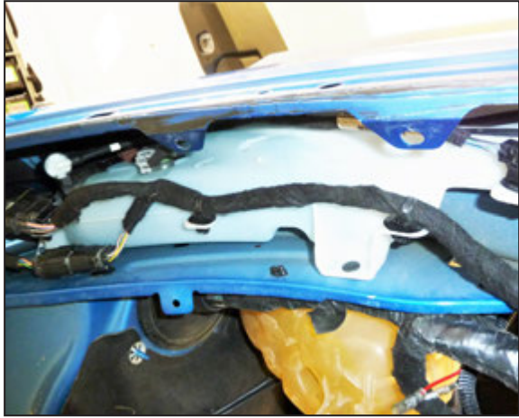
25. Reinstall the windshield washer bottle using the factory hardware. Secure the wiring harness to the bottle. Reinstall the filler neck using the factory hardware.
