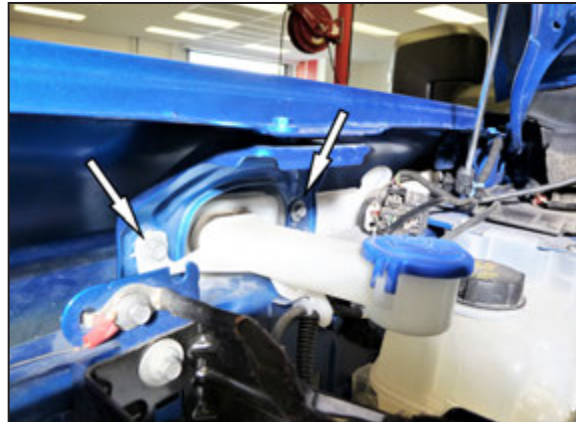
5. Remove the two bolts that secure the windshield washer bottle filler neck and remove the filler neck from the vehicle. NOTE: Some washer fluid may come out, keep a towel handy.
