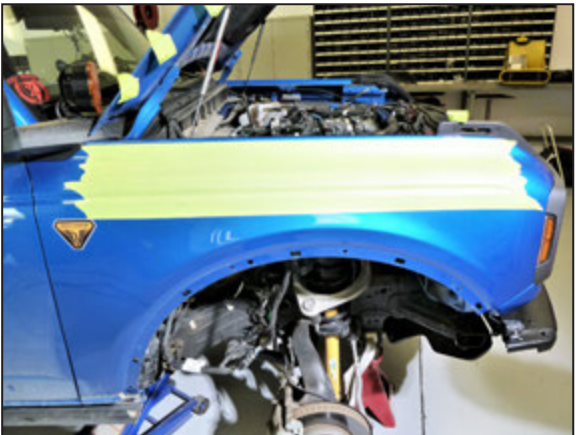
10. Apply painters' tape to the fender to protect the surrounding paint while drilling holes.
