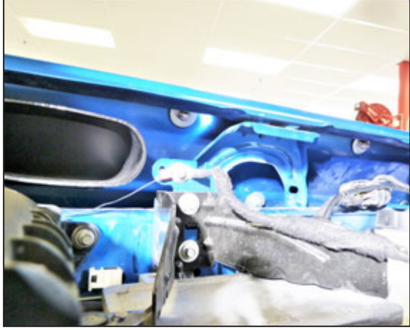
22. Install the three nuts onto the mounting studs along with the fender washers. Do not tighten the nuts.
