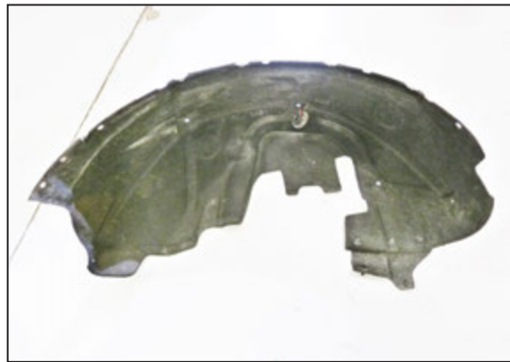
4. Remove the fasteners that secure the inner fender and then remove the inner fender from the vehicle.
