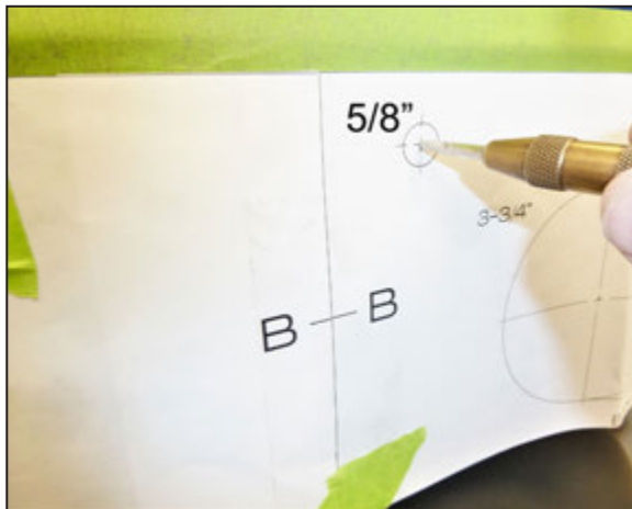
12. Using a punch, mark the seven locations to be drilled.
