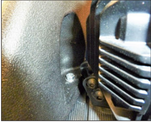
24. Install the provided 6mm bolt thru the snorkel into the cowl/mirror mount. Tighten all the mounting hardware.
