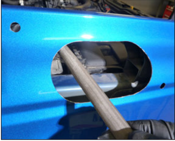
17. Deburr the holes with a file or similar device.
