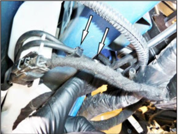
7. Disconnect the windshield washer hose at the union fitting and then unhook the mount from the inner fender.
