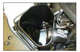
8. Install the K&N air filter housing assembly into the vehicle so the mounting studs insert into the factory grommets.
