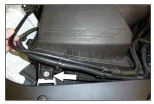
4. Unhook the coolant line and wiring harness from the air filter housing. Remove the bolt securing the air filter housing to the core support and then remove the intake system from the vehicle.
