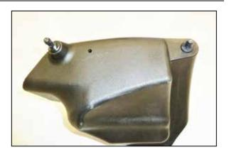
5. Install the provided mounting posts onto the K&N air filter housing using the provided hardware.
