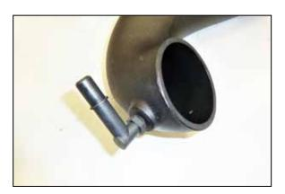
11. Install the provided quick connect fitting into the K&N intake tube as shown.
