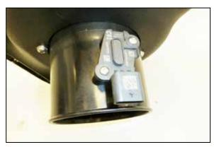
7. Remove the mass air sensor from the factory housing and install it into the K&N housing using the provided hardware.
