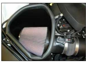
14. Install the provided edge trim onto the top of the air filter housing as shown. Some trimming of excess edge trim will be necessary.
