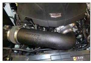
12.Install the K&N intake tube into the hump coupler and then into the coupler at the throttle body, adjust for best fit and then secure with the provided hose clamps.
