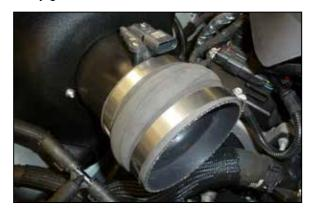
9.Install the hump coupler onto the mass air sensor housing and secure with the provided hose clamp.
