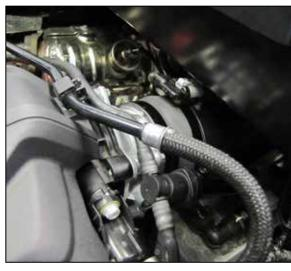
31. Reconnect the mass air sensor electrical connection.
