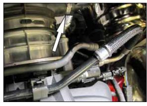
11. Cut the one time use clamp that secures the CCV hose and then disconnect the CCV hose from the factory intake tube. Loosen the hose clamp that secures the intake tube to the throttle body.
