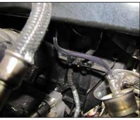
13. Disconnect the wiring harness's that attach to the rear of the air filter assembly.
