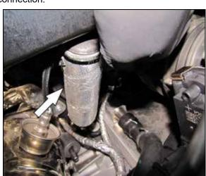
9. Disconnect the transmission vent canister from the air filter housing.
