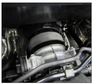
30. Insert the intake tube into the coupler at the throttle body and secure with the provided hose clamp. Be sure the tube and filter are aligned and straight before tightening the holes clamps.
