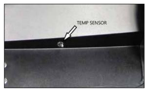
24a. Attach the air temperature sensor from step #23 through the hole on the bottom of the passenger side heat shield on the engine side.
