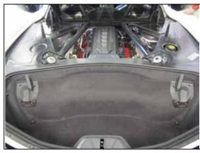
32. Reinstall the filter access panel, carpet and top stowage mounts using the factory hardware.
