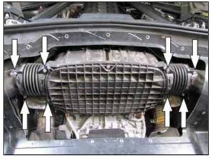
5. Remove the eight bolts that secure the two fresh air intake ducts and then remove the two ducts. These ducts will not be reused.
