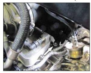
12. Remove the driver's side lower air box mounting bolt.
