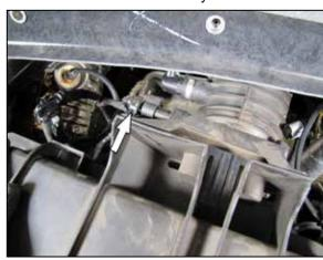
14. Pull the air filter assembly back slightly to expose "F" antenna at the top of the housing. Disconnect the electrical connection of the "F" antenna and then remove the air filter assembly from the vehicle. Remove the two fresh air duct extensions from the vehicle. These ducts will not be reused.
