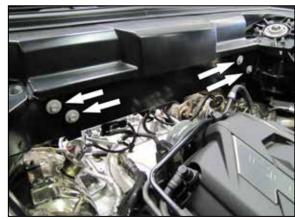
15. Install the two-heat shield mounting brackets to the chassis cross member using the four-air box mounting bolts.
