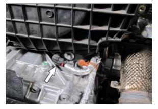
6. Disconnect the air temperature sensor electrical connection.
