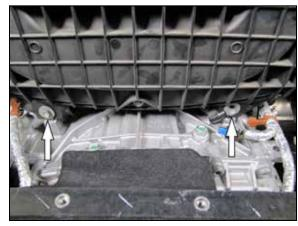
7. Remove the two bolts that secure the bottom of the air box.
