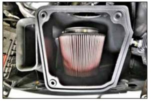
8. Set the K&N air filter into the filter housing.
