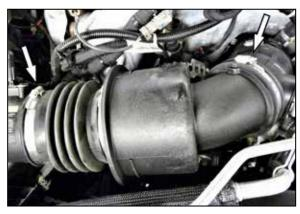
2. Loosen the two hose clamps securing the factory intake hose and then remove the hose from the vehicle.
