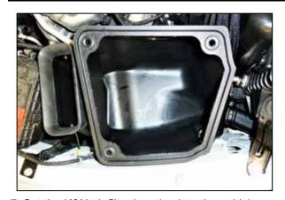
7. Set the K&N air filter housing into the vehicle so the studs protrude into the factory mounting grommets. Secure the K&N Air filter housing with the facory from step #4.
