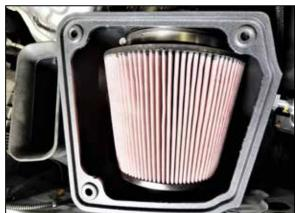
10. Slide the K&N air filter onto the filter adapter and secure with the provided hose clamp.
