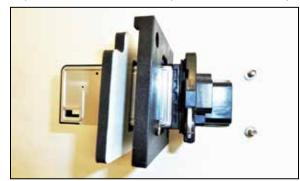
13. Remove the mass air sensor from the factory air filter housing. Assemble the mass air sensor, adapter and gasket as shown. NOTE: 2024 model year vehicles and later have a different mass air sensor, the connector lays flat as compared to the sensor pictured.
