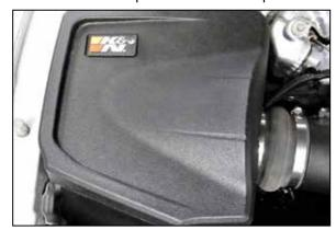
11. Install the K&N badge onto the lid and then install the lid onto the air filter housing as shown.
