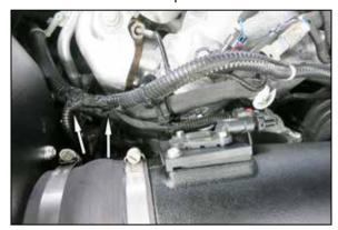
16. On 2024 and later model year vehicles that the electrical connection lays flat, it will be necessary to cut the electrical tape that secures the MAF pigtail to the main harness. Then pull approximately two inches of the MAF pigtail harness out from the main harness and retape the harness covering This will allow enough slack in the harness to allow connection.
