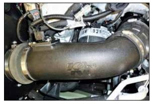
15. Install the K&N intake tube assembly into the coupler at the filter adapter and then into the factory coupler, adjust the tube for best fit and secure with the hose clamps.
