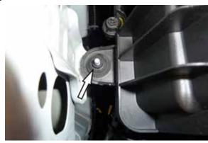
4. Remove the nut that secures the air filter housing into the vehicle and then lift up and remove the air filter housing from the vehicle.
