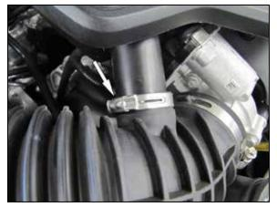
3. Prv loose the band clamp that secures the intake plenum tube to the intake hose and remove the
