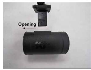
11. Remove the mass air sensor from the factory housing. Install the mass air sensor into the adapter provided and secure with the provided hardware. Install the provided gasket onto the adapter and then install the assembly into the K&N® intake tube and secure with the provided hardware. NOTE: Be sure to install the sensor assembly in the direction shown, the open end of the sensor is to be towards the air filter.
