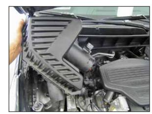
5. Pull up the factory air filter housing to dislodge it from the mounting grommets and then remove the housing from the vehicle. NOTE: K&N Engineering, Inc., recommends that customers do not discard factory air intake.
