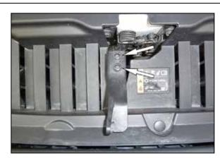
5. Remove the two bolts that secure the hood release arm to the hood latch and then remove the arm
