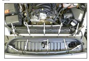
6. Release the ten retaining clips that secure the upper radiator valence and then remove the valence from the vehicle.
