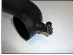
20.Install the provided  $90^{\circ}$  quick connect fitting into the K&N® intake tube as shown.
