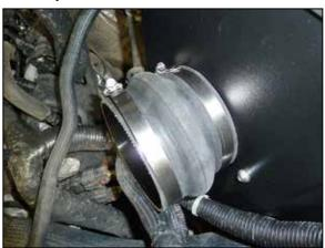
18. Install the provided hump coupler onto the filter adapter and secure with the provided hose clamp.
