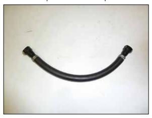
24. Install the provided quick connect fittings into the provided crank case vent hose and secure with the provided hose clamps.
