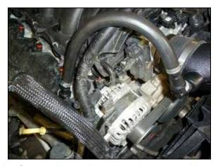
25. Connect the crank case vent hose assembly to the valve cover port and then to the fitting installed into the intake tube.
