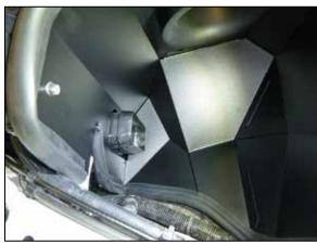
14. Install the heat shield assembly into the vehicle so the mounting grommet slides into the factory mounting hole. Slide the fresh air intake scoop into the opening in the heat shield and resecure to the core support with the factory clip. Secure the heat shield with the factory nut removed in step #9.
