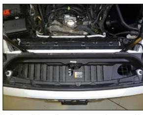
16. Reinstall the radiator valence and secure with the ten factory clips.
