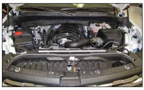
28. Reinstall the upper radiator valence and secure with the factory retaining clips.
