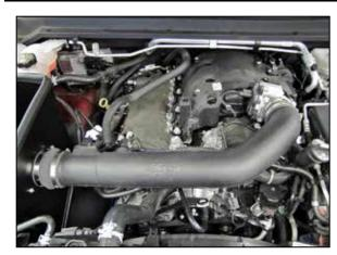
18. Install the provided hump coupler (08699) onto the K&N® intake tube, then install the intake tube assembly into the coupler at the throttle body and align with the filter adapter. Slide the hump coupler onto the filter adapter, adjust the tube for best fit and secure with the provided hose clamps.
