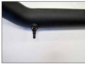
17. Install the quick connect fitting into the  $K\&N^{\otimes}$  intake tube as shown.
