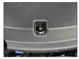
4. Remove the front center bolt securing the intake plenum to the engine and remove the intake plenum from the vehicle.
