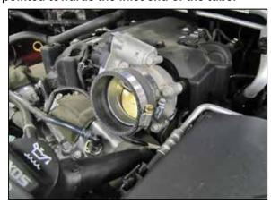
15. Install the provided coupler (08186) onto the throttle body and secure with the provided hose clamp.
