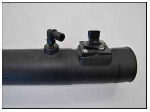
16. Install the  $90^{\circ}$  vent fitting into the K&N® intake tube as shown.
