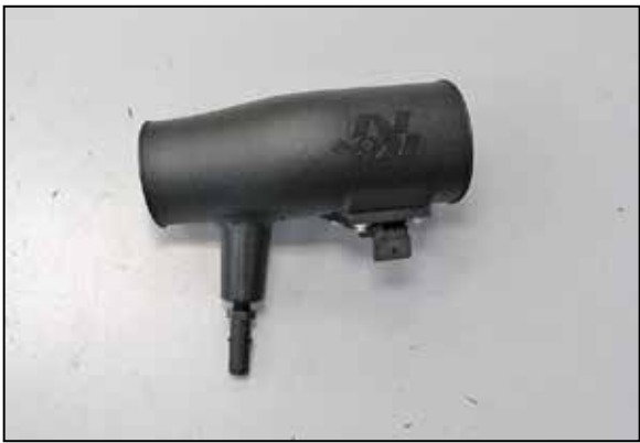
18. Install the Provided NPT quick disconnect fitting into the K&N® intake tube as shown. NOTE: NPT fittings are easy to cross thread. Install the vent fitting "hand" tight, then turn it two complete turns with a wrench.
