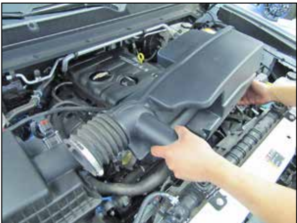
5. Remove the intake plenum from the vehicle.
