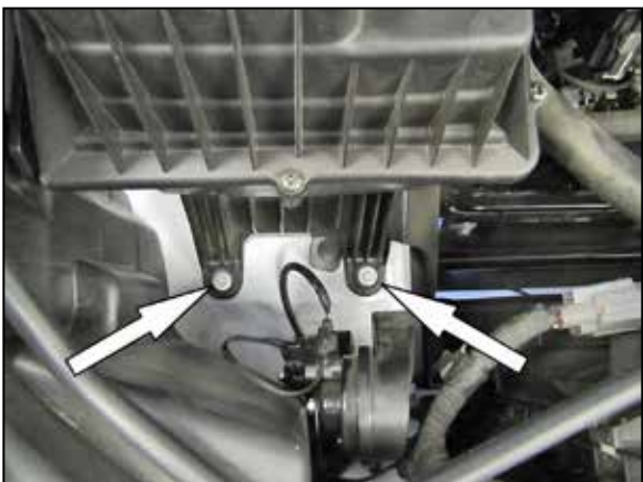
7. Remove the two bolts securing the air filter housing to the inner fender. NOTE: One of the nuts will be reused in a later step.
