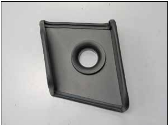
11. Install the edge trim onto the heat shield as shown. NOTE: Some trimming of the edge trim will be necessary.
