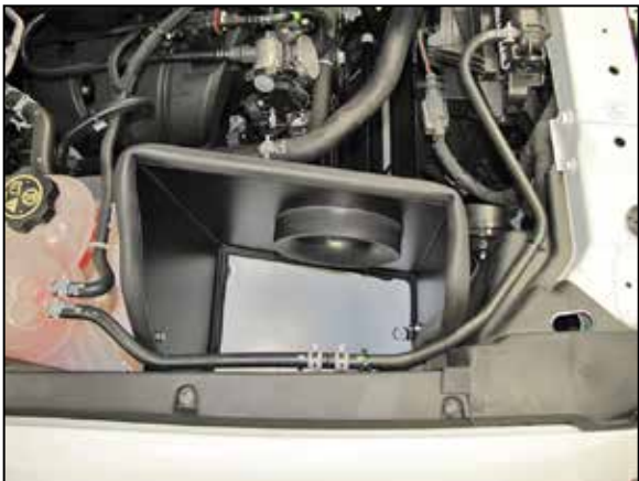
14. Install the heat shield into position and secure with the two of the factory nuts removed in earlier steps.
