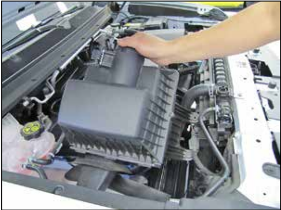
8. Remove the air filter housing assembly from the vehicle. NOTE: K&N Engineering, Inc., recommends that customers do not discard factory air intake.
