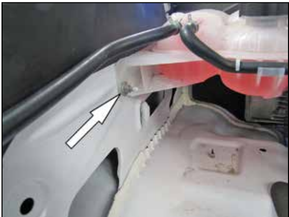
9. Remove the nut securing the coolant reservoir to the inner fender. NOTE: This nut will be reused in a later step.
