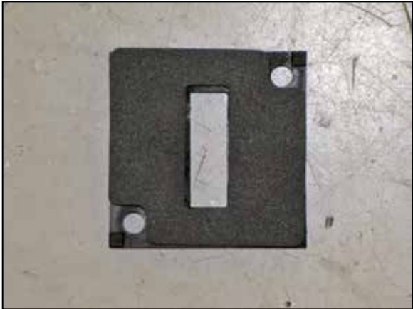
15. Install the provided gasket onto the K&N® mass air sensor adapter.
