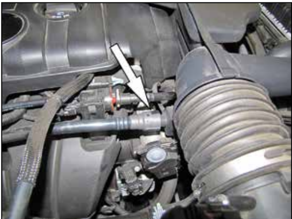
4. Disconnect the crank case vent hose from the intake plenum.
