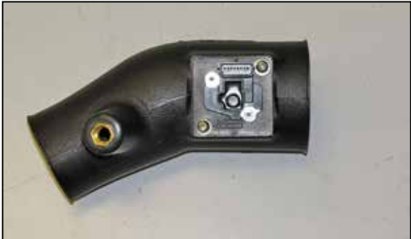
17. Install the mass air sensor into the K&N® adapter and then install the assembly into the K&N® intake tube and secure with the provided hardware. NOTE: be sure to install the sensor in the correct position. The opening in the sensor is to be pointed towards the air filter end of the tube.
