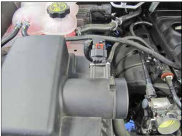
6. Disconnect the mass air sensor electrical connection.
