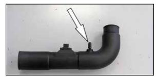
17. Install the vent fitting into the K&N® intake tube. NOTE: NPT fitting has tapered threads and only designed to be installed until hand tight, then tighten one rotation or when the fitting becomes difficult to return.
