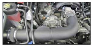
18. Install the K&N® intake tube into the hose at the filter adapter and then into the hose at the throttle body. Adjust the tube for best fit and then secure with the provided hose clamps.
