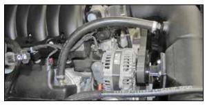
19. Install the provided crank case vent hose onto the valve cover port and onto the vent installed into the intake tube. Secure the hose with the provided hose clamps.
