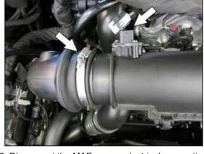
2. Disconnect the MAF sensor electrical connection and then loosen the hose clamp that secures the factory intake tube to the air filter housing.
