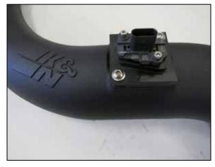
9. Remove the MAF sensor from the factory air filter housing and then install it into the K&N intake tube using the provided Adapter, Gasket & hardware as shown.
