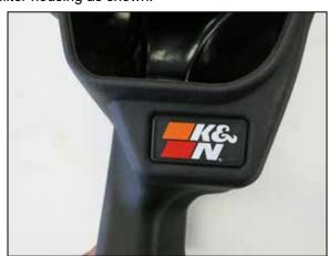
12. Install the K&N badge into the K&N air filter housing as shown.
