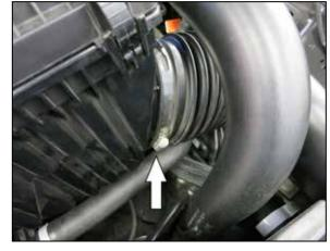
3. Loosen the hose clamp that secures the fresh air duct to the air filter housing.
