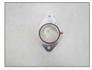
13. Remove the sealing O-ring from the factory turbo flange and install it into the K&N turbo flange.
