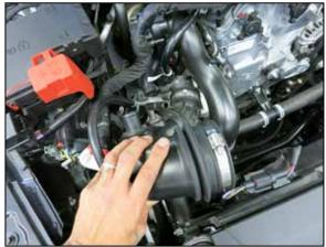
7. Remove the intake tube from the vehicle.
