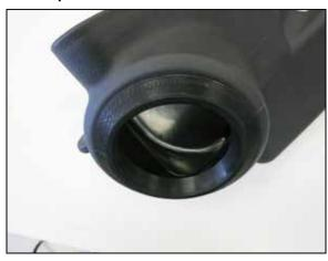
11. Install the provided tube seal into the K&N air filter housing as shown.
