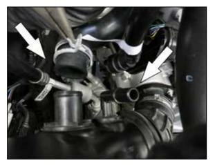
5. Disconnect the BOV hose and the CCV hose from the factory intake tube.
