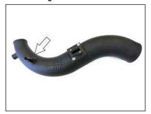
10. Install the provided CCV quick connect fitting into the K&N intake tube as shown.
