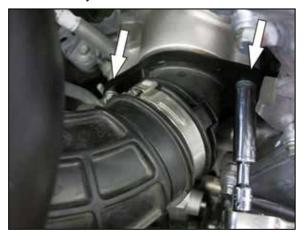
6. Remove the two nuts that secures the turbo inlet onto the turbo.
