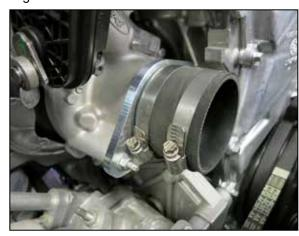
15. Install the turbo flange assembly onto the turbo and secure with the factory hardware.
