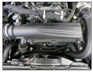
4. Remove the two mounting nuts, disconnect the intake & fresh air hoses and remove the factory air filter housing. Remove the fresh air scoop.
