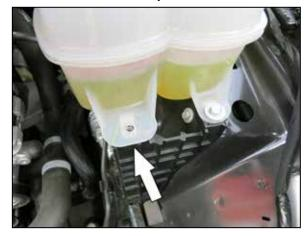
16.Remove the coolant bottle mounting bolt shown.
