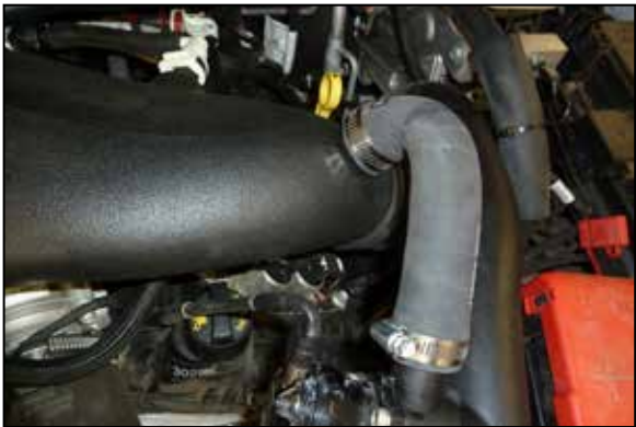
28. Install the provided BOV hose and secure with the provided hose clamps.
