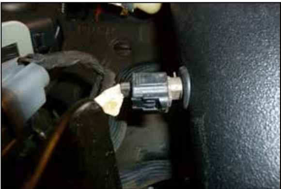
22. Reconnect the IAT sensor electrical connection.
