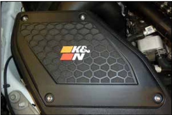
24. Assemble the filter housing lid and install it onto the K&N air filter housing using the provided hardware.
