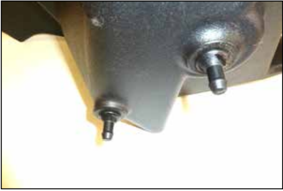
18. Install the mounting studs onto the K&N air filter housing using the provided hardware.
