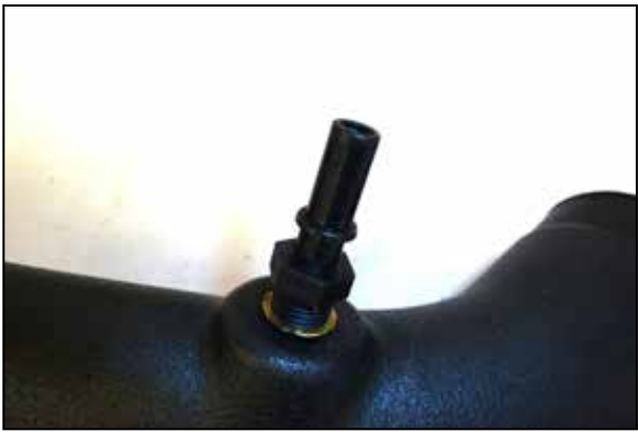
13. Install the provided quick connect fitting into the K&N intake tube.
