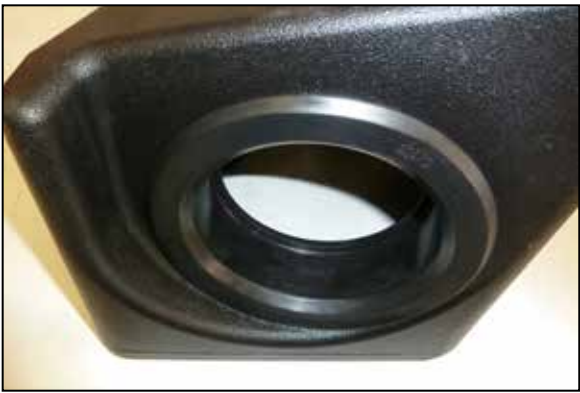
17. Install the tube adapter into the K&N air filter housing.
