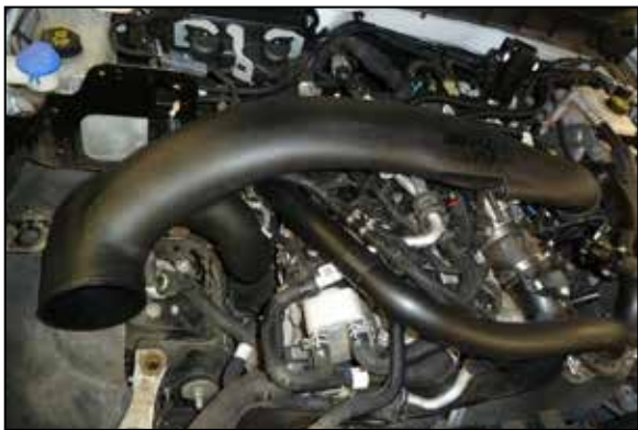
16. Install the K&N intake tube into the factory driver side coupler and then into the coupler installed onto the passenger side turbo. Do not tighten the hose clamps.
