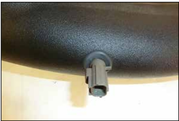
15. Remove the IAT sensor from the factory intake tube, remove the O-ring from the sensor and then install the sensor into the K&N intake tube using the provided grommet. NOTE: Use care while handling the IAT sensor as it is very fragile.
