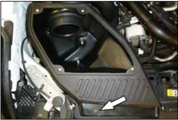
19. Install the K&N air filter housing into the vehicle. While installing the housing, insert the intake tube into the adapter installed into the housing. Push the housing down so the mounting pins insert into the factory mounting grommets and then reinstall the factory pin to secure the fresh air duct to the core support.
