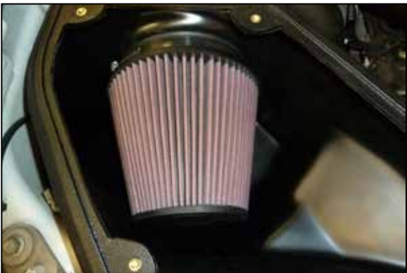
23. Install the K&N air filter onto the filter adapter and secure with the provided hose clamp.
