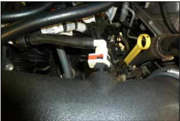
26. Connect the rear vent line to the quick connect fitting installed into the K&N intake tube.
