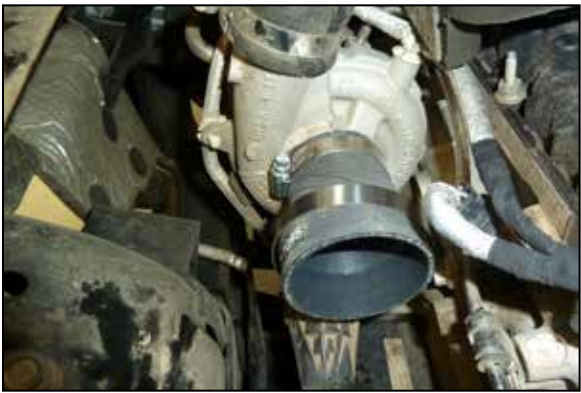
12. Install the provided step coupler onto the passenger side turbo and secure with the provided hose clamp.
