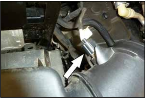
7. Disconnect the IAT sensor electrical connection.
