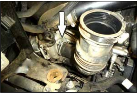
10. Release the spring clamp that secures passenger side intake tube to the turbo and then remove the tube from the vehicle.
