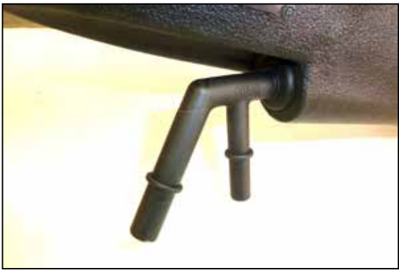
14. Install the provided Ejector fitting into the K&N intake tube with the provided grommet.
