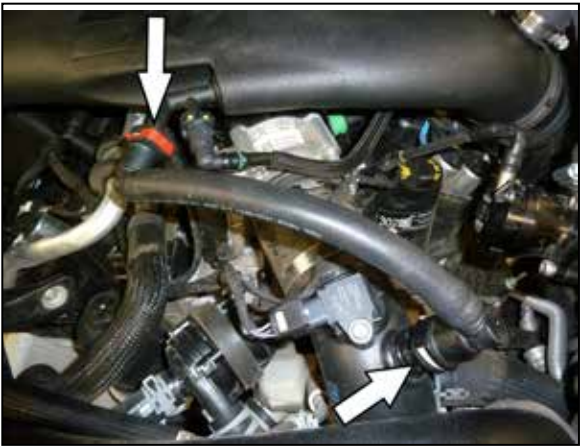
25. Connect the smaller vent line to the Ejector fitting installed into the K&N intake tube. Remove the two fittings from the larger factory vent line and install them into the vent hose provided. NOTE: Use a heat gun or hair drier to heat the vinyl line and ease the removal of the fittings from the factory line.
