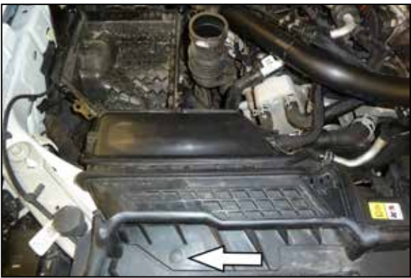
9. Remove the plastic hold-down clip that secures the fresh air duct to the core support, then lift the lower housing up and remove it from the vehicle.
