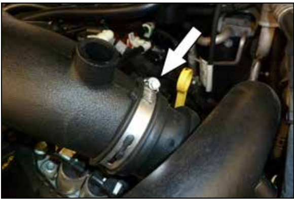
21. Tighten the hose clamp the secures the intake tube to the driver side turbo coupler.
