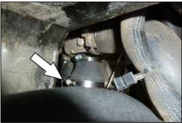
20. Align the intake tube for best fit and then tighten the hose clamp at the passenger side turbo.
