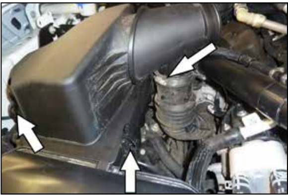
8. Loosen the hose clamp that secures the passenger side intake tube to the air filter housing, release the clamps that secure the air filter housing lid to the lower housing and then remove the upper housing lid and filter from the vehicle.
