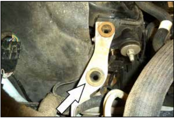
11. Remove the upper air filter housing mounting grommet and install in the location shown.
