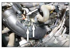
9. Release the locks that secure the vent lines to the ejector fitting and CCV fitting, then disconnect the lines from the fittings.
