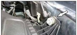
3. Remove the bolt that secures the air filter housing to the inner fender and the two retaining pins securing the fresh air duct then lift the air filter housing up to dislodge it from the mounting grommets and remove it from the vehicle.
