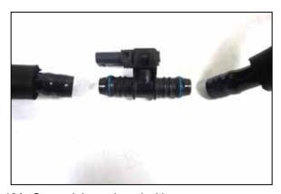
18A. On models equipped with a pressure sensor in the CCV line, pull back the outer foam covering and then use a heat gun or similar source, warm the CCV line enough to release the connection to the pressure sensor. Disconnect the CCV lines from the pressure sensor.
