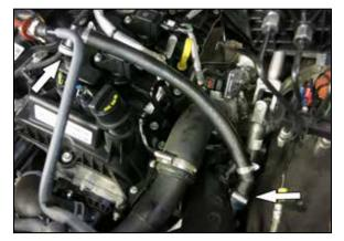
19. Now install the CCV hose assembly into vehicle and connect to engine and inlet tube. NOTE: On models equipped with a pressure sensor in the CCV line, reconnect the pressure sensor electrical connection.
