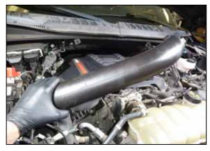
5. Dislodge the passenger side turbo inlet tube from the mounting grommet and then remove it from the vehicle.
