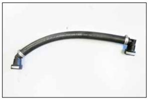
18. Remove the factory CCV line from the valve cover. Assemble the provided CCV hose assembly as shown with the hardware provided. NOTE: Some vehicles may be equipped with a pressure sensor in the CCV line. See Steps 18A & 18B.
