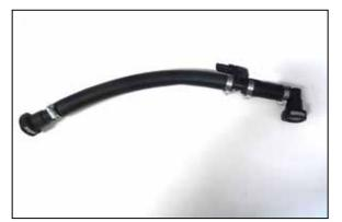
18B. Measure back three inches from the 90-degree quick connector and then cut out a oneinch section of hose. Install the pressure sensor from the previous step as shown and secure with the provided hose clamps.
