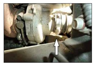
4. Loosen the hose clamp for the passenger side turbo inlet tube by accessing the hose clamp on the turbo inlet through the passenger side wheel well. Lift the splash shield up and use a ratchet, extension with 7mm socket.
