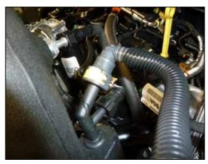
21. Connect the vent lines to the quick connect fitting and ejector fitting.
