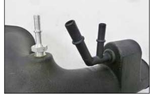
16. Install the quick connect fitting into the driver side upper K&N intake tube. Install the provided ejector fitting with the provided grommet into the intake tube. NOTE: When installing the ejector fitting, grab it on the main shaft not the extended portion to prevent possible breakage. NOTE: Some later models may not have the single quick disconnect vent line, in this case install the provided 1/4"NPT plug into the intake tube.
