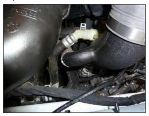
15. Connect the BOV hose to the K&N lower intake tube. *NOTE: On vehicles not equipped with a BOV, skip to the next step.*
