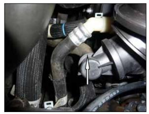
6. Release the BOV hose spring clamp and then disconnect and remove the BOV hose. **NOTE:**Some models may not be equipped with a BOV, on these models skip to next step.
