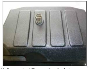
10. Remove the IAT sensor from the factory upper air filter housing, remove the O-ring from the sensor and then install it into the K&N air filter housing using the provided grommet.
