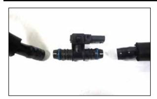
17A. On models equipped with a pressure sensor in the CCV line, pull back the outer foam covering and then use a heat gun or similar source, warm the CCV line enough to release the connection to the pressure sensor. Disconnect the CCV lines from the pressure sensor.
