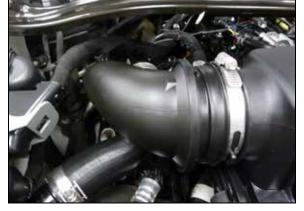
2. Loosen the hose clamps that secure the passenger side intake tube to the turbo inlet and factory air filter housing. Remove the passenger side intake tube from the vehicle.
