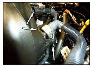
3. Depress the locking tabs and then disconnect the three vent lines attached to the driver side intake tube.
