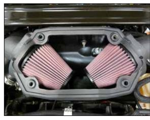
25. Install the air filters onto the intake tube and secure with the provided hose clamps. Install the four grommets into the lid mounting holes in the air filter housing.
