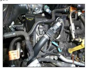
18A. On models equipped with the pressure sensor in the CCV line, reconnect the pressure sensor electrical connection.
