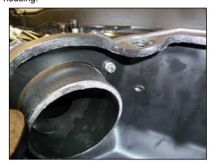
24. Secure the intake tube to the K&N air filter housing using the provided hardware.
