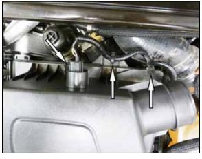
8. Disconnect the IAT sensor electrical connection and unhook the wiring harness from the air filter housing, release the over center clips and then remove the upper air filter housing and filter.
