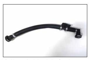
17B. Measure back three inches from the 90-degree quick connector and then cut out a oneinch section of hose. Install the pressure sensor from the previous step as shown and secure with the provided hose clamps.
