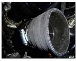
22. Install the provided coupler onto the passenger side turbo inlet.
