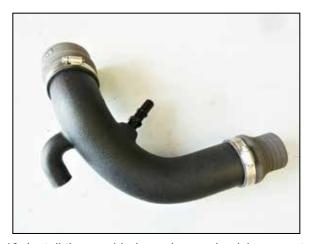
13. Install the provided couplers and quick connect fitting into the lower driver side intake tube. **NOTE:** on models that do not have a BOV, install the provided CAP onto the fitting molded into the K&N intake tube and secure with the provided hose clamp. The cap is a tight fit.
