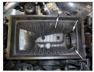
9. Remove the lower air box mounting nut. Release the three locking tabs that secure the fresh air intake duct and the unhook the duct from the lower air filter housing. **NOTE: K&N Engineering, Inc., recommends that customers do not discard factory air intake.**
