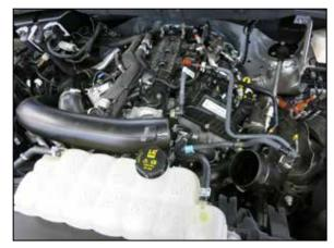
4. Dislodge the passenger side turbo inlet tube from the mounting grommet and then remove it from the vehicle.
