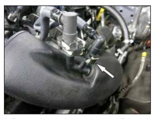
21. Connect the vent lines to the ejector fitting installed into the K&N inlet tube.
