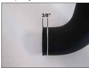
6a. On 2023 and later Ford Raptor model vehicles it is necessary to trim 3/8" off the end of tube p/n 087545. Using a marker, measure and draw a line 3/8" from the turbo inlet end of the tube as shown.
