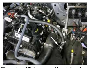
20. Install the CCV hose assembly onto the valve cover and turbo inlet tube fittings. NOTE: On models equipped with the pressure sensor in the CCV line, reconnect the pressure sensor electrical connection.
