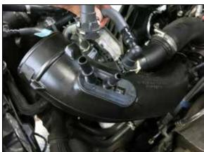
8. Release the locks that secure the vent lines to the ejector fittings and then disconnect the lines from the fittings.
