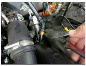
10. Using a pair of side cutters, cut the black hard-shell portion of the CCV connectors at the valve cover and turbo inlet tube so the fittings can be disconnected and the CCV hose assembly and be removed. NOTE: Some vehicles may be equipped with a pressure sensor in the CCV line, Disconnect the pressure sensor electrical connection at this time.
