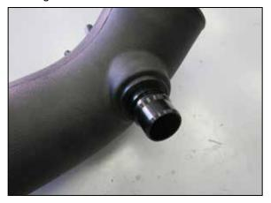
15. Install the grommet and BOV fitting into the driver side K&N turbo inlet tube. Apply a small amount of lubricant onto the fitting to ease installation.
