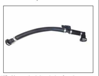
19B. Measure back three inches from the 90-degree quick connector and then cut out a one-inch section of hose. Install the pressure sensor from the previous step as shown and secure with the provided hose clamps.
