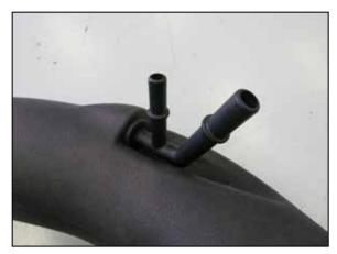
14. Install the provided ejector fitting into the K&N driver side turbo inlet tube using the provided grommet. **NOTE**: The ejector fitting is fragile, Grab the fitting on the main body and use a twisting motion while pushing the fitting into the grommet. Using some lubricant like WD40 will ease the installation into the grommet. Pushing in the fitting on the top vent leg may result in the fitting fracturing.
