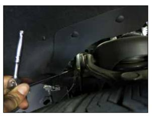
3. Remove the passenger side turbo inlet tube by accessing the hose clamp on the turbo inlet through the passenger side wheel well. Lift the splash shield up and use a ratchet, extension with 7mm socket.
