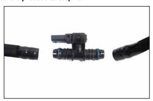
19A. On models equipped with a pressure sensor in the CCV line, use a heat gun or similar source, warm the CCV line enough to release the connection to the pressure sensor. Disconnect the CCV lines from the pressure sensor.
