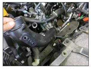
11. Loosen the hose clamp at the turbo inlet, unhook the mounting post and remove the driver side turbo inlet tube.
