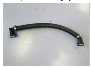
19. Assemble the provided CCV hose as shown. NOTE: On models equipped with a pressure sensor in the CCV line go to step #19a, all others proceed to step 20.
