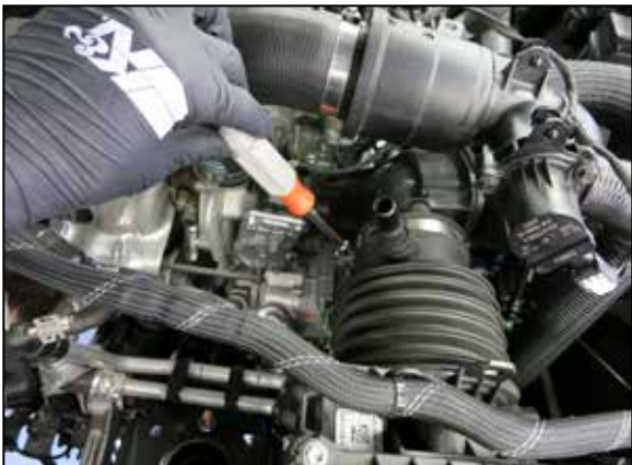
4. Loosen the hose clamp that secures the factory intake tube connection shown.
