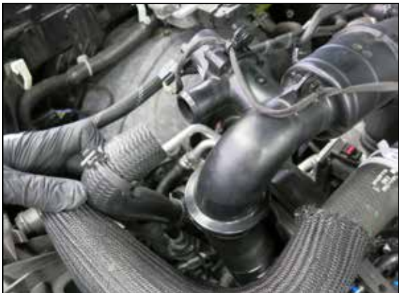
10. Release the spring clamp that secures the BOV hose to the fitting and then disconnect the hose.
