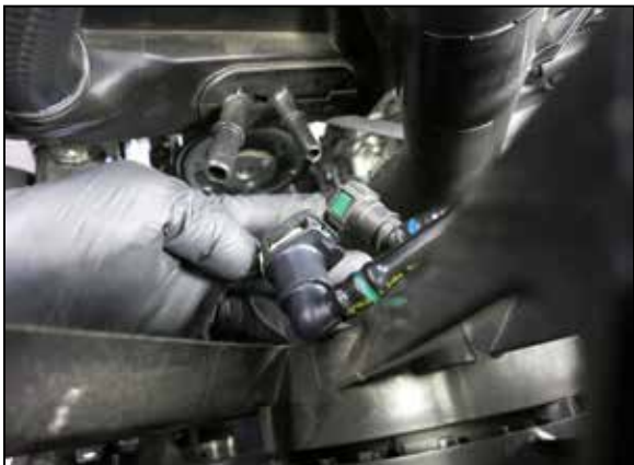
12. Depress the green locking clip on the smaller EVAP hose and then disconnect it from the ejector fitting.
