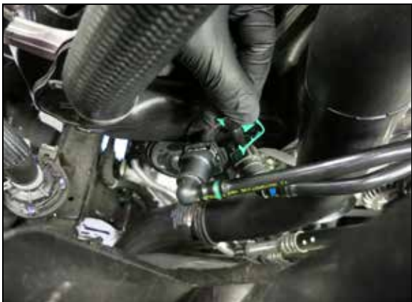
11. Remove the green locking clip that secures the larger EVAP hose to the Ejector fitting and then disconnect the hose.
