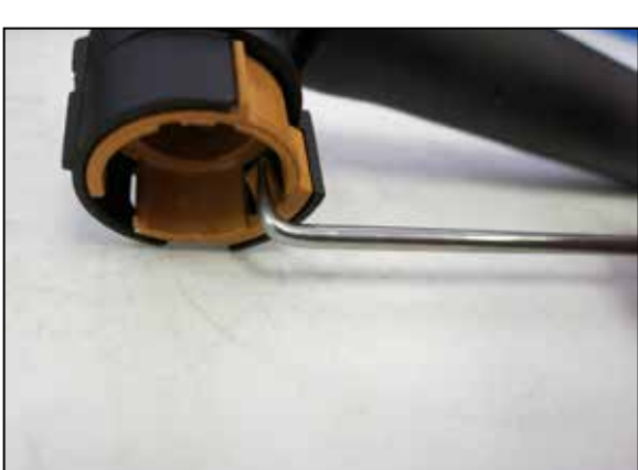
13. Disconnect the CCV hose from the valve cover. There are three clips inside the connector that lock the fitting onto the valve cover, using a 90degree pick the clips can be released one at a time while applying slight pressure upwards on the fitting. The upward pressure will help prevent the clips from relocking while releasing the others. Replacement connectors are provided to be used with the K&N intake kit.
