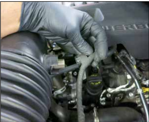
3. Disconnect the IAT sensor electrical connection.
