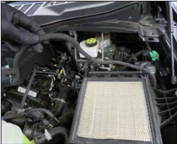
6. Unhook the IAT sensor wiring harness from the lower air filter housing.
