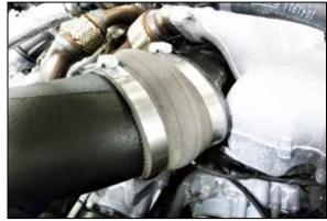
16. Slide the hump coupler onto the turbo inlet pipe and then secure with the provided hose clamps.
