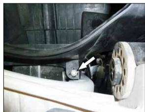
6. Remove the bolt securing the air filter housing and then remove the housing from the vehicle. NOTE: K&N Engineering, Inc., recommends that customers do not discard factory air intake.
