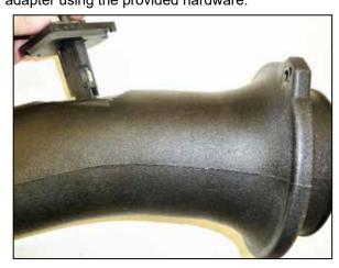
11. Install the mass sensor assembly into the K&N intake tube, be sure to install the sensor in the correct position so the opening of the sensor is pointed towards the filter end of the intake tube.
