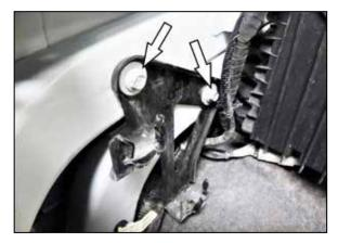
7. Remove the two bolts securing the air filter housing bracket to the inner fender and then remove the bracket from the vehicle.
