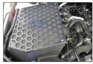
16. Install the filter lid assembly onto the air filter housing and secure with the provided hardware.
