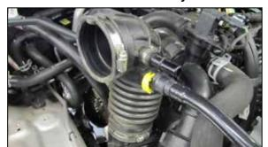
7. Loosen the hose clamp that secures the intake hose to the plenum and then remove the hose from the vehicle.
