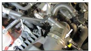
5. Remove the rear air filter housing mounting bolt and loosen the hose clamp that secures the intake hose to the housing.
