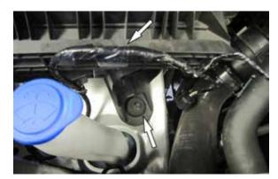
4. Remove the front air filter housing mounting bolt and unhook the wiring harness from the housing.
