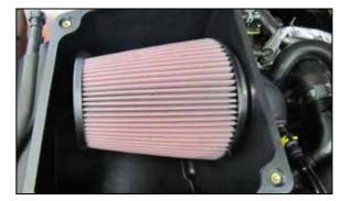
15. Install the K&N air filter onto the filter adapter and secure with the provided hose clamp.
