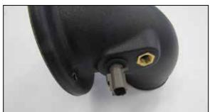
9. Remove the inlet air temperature sensor from the factory housing. Remove the O-Ring from the sensor and then install the sensor into the K&N intake tube using the provided grommet.
