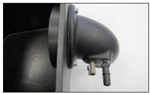
11.Install the bolts and washers into the intake tube, then install the gasket. Now install the tube assembly onto the air box so the bolts pass through the three holes, then install the second gasket and filter adapter. Secure the complete assembly with the provided hardware.
