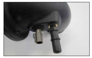
10. Install the provided crank case quick connect fitting into the K&N intake tube as shown. NOTE: NPT fittings are easy to cross thread. Install the vent fitting "hand" tight, then turn it two complete turns with a wrench.
