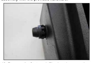
12. Remove the factory air filter housing mounting post and install it onto the K&N air filter housing as shown.
