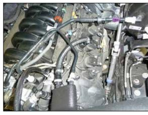
25. Connect the 90° fitting to the valve cover and the straight fitting to the fitting installed into the K&N® intake tube. Connect the EVAP vent line to the fitting installed into the K&N® intake tube.
