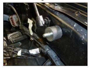
10. Install the provided rubber mounted stud into the factory air filter housing mounting location on the inner fender.
