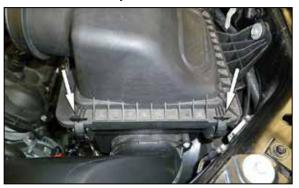
6. Release the two locking clips that secure the upper air filter housing and then remove the upper housing from the vehicle.
