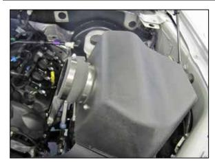
19. Install the provided hump coupler (08639) onto the filter adapter and secure with the provided hose
