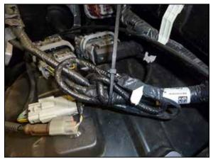
9. On vehicles that have the wiring pig tail that was attached to the lower air filter housing, use the provided tie wrap and secure the pig tail back away from the air filter housing location.
