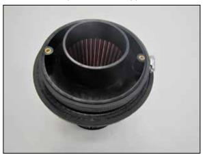
16. Install the K&N® air filter onto the filter adapter and secure with the provided hardware.
