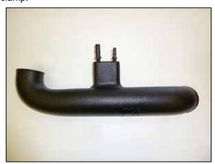
21. Install the provided vent fittings into the K&N® intake tube as shown.
