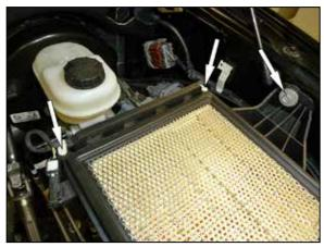
8. On vehicles equipped with the wiring pigtail that secures to the lower air filter housing, disconnect the wiring harness from the lower air filter housing. Remove the bolt that secures the lower air filter housing to the inner fender and then remove the lower housing from the vehicle.
