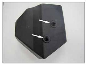
11. Install the two provided mounting studs onto the K&N® filter housing using the provided hardware.
