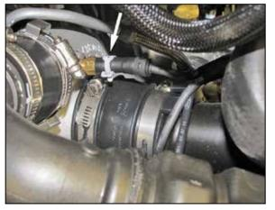
5. Loosen the hose clamp securing the intake tube to the Turbo.
