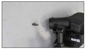
16. Remove the inlet air temperature sensor from the factory air filter housing.
