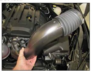
6. Remove the factory intake tube from the vehicle. NOTE: K&N Engineering, Inc., recommends that customers do not discard factory air intake.
