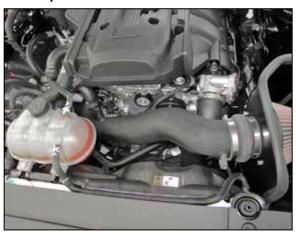
20. Slide the provided hump hose (08418) onto the end of the K&N® intake tube, then install the intake tube into the hose at the turbo inlet. Slide the hump hose into position on the filter adapter and secure the tube with the provided hose clamps.
