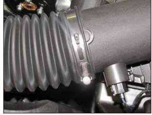
2. Loosen the hose clamp securing the factory intake tube to the air filter housing.
