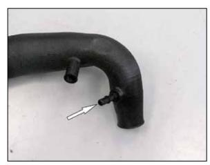
19. Install the provided quick disconnect fitting into the K&N® intake tube as shown.
