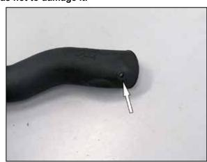
17. Install the provided grommet into the  $K\&N^{\scriptsize @}$  intake tube as shown.
