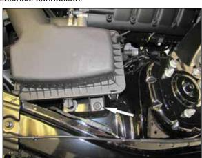
8. Remove the bolt securing the air filter housing to the inner fender and remove the air filter housing from the vehicle
