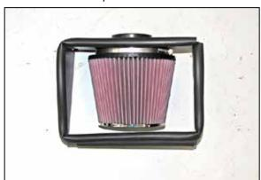
10. Install the K&N® air filter onto the filter adapter and secure with the provided hose clamp.
