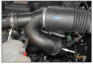
5. Loosen the two hose clamps that secure the factory intake tube to the turbo inlets, then remove the factory intake tube from the vehicle.
