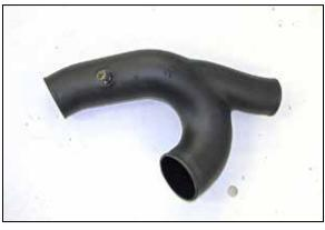
16. Remove the O-Ring from the inlet air temperature sensor, then install it into the grommet installed into the K&N® intake tube.
