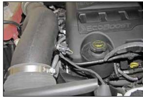
18. Reconnect the inlet air temperature sensor electrical connection using the provided extension harness.
