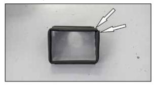
8. Install the provided bulb edge trim onto the top of the heat shield as shown.
