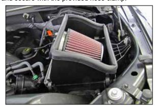
11. Install the heat shield/filter assembly onto the factory lower air filter housing and secure with the factory retaining clips.
