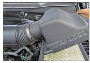
4. Release the locking clips that secure the upper air filter housing to the lower housing, then lift the upper housing and remove it from the vehicle. Remove the factory air filter from the vehicle.
