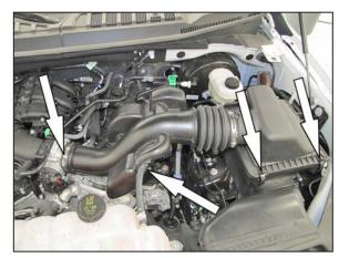
4. Loosen the hose clamp securing the intake tube to the throttle body, unhook the coolant reservoir hose from the intake tube and unclip the two upper air filter housing retaining clips. Then remove the upper air filter housing and intake tube assembly. NOTE: K&N Engineering, Inc., recommends that customers do not discard factory air intake.
