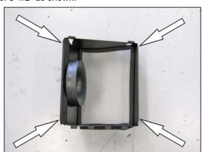
8. Install the two small edge trim onto the bottom of the heat shield as shown.
