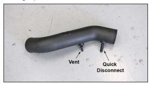
11. Install the provided NPT quick disconnect fitting and NPT vent fitting into the K&N® intake tube as
