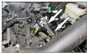
17. Install the quick disconnect union into the mating EVAP quick disconnect fitting and then connect the open EVAP vent hose to the fitting installed into the K&N® intake tube.
