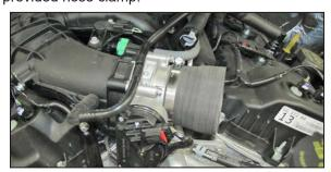
13. Install the provided step coupler hose (084055) onto the throttle body and secure with the provided hose clamp.
