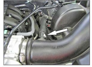
2. Disconnect the Crank case vent hose quick connect fitting.
