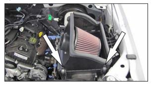
10. Install the heat shield assembly onto the lower air filter housing and secure with the factory retaining clips.
