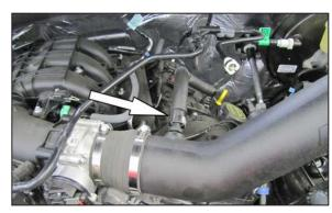
15. Connect the crank case vent quick disconnect fitting to the mating quick disconnect fitting installed into the K&N® intake tube.
