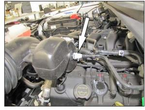
3. Disconnect the EVAP vent quick connect fitting.
