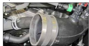
14. Install the provided coupling hose (08761) onto the driver's side turbo inlet tube and secure with the provided hose clamp.
