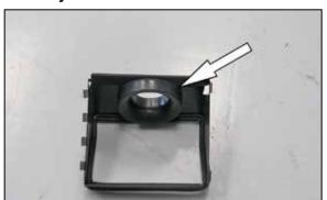
10. Install the provided filter adapter into the heat shield and secure with the provided hardware.
