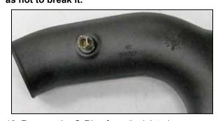
18. Remove the O-Ring from the inlet air temperature sensor, then install it into the grommet installed into the K&N® intake tube.
