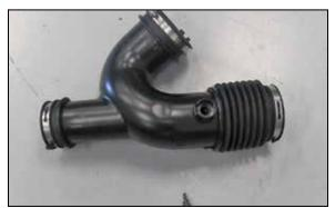
17. Unlock the inlet air temperature sensor and rotate it counter clockwise, remove the sensor from the factory air filter housing.
