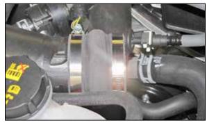
15. Install the provided coupling hose (087121) onto the passenger side turbo inlet tube and secure with the provided hose clamp.
