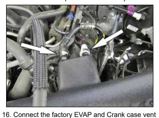
lines to the fittings on the K&N® intake tube.
