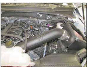
15. Install the K&N® intake tube into the coupling hose at the filter adapter and then into the hose at the throttle body, adjust the tube for best fit and then secure with the provided hose clamps.
