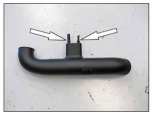
14. Install the two provided quick disconnect fittings into the K&N® intake tube as shown.
