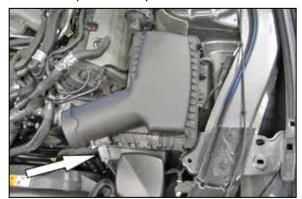
8. Release the locking tab and then disconnect the mass air sensor electrical connection.
