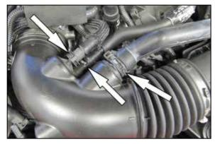
4. Depress the locking tabs and then disconnect the crank case vent hose and the EVAP vent hose. Then release the spring clamp and disconnect the sound tube from the intake tube.
