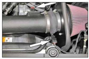
26. Connect the provided mass air sensor extension harness into the factory mass air sensor connection and then connect the other end to the mass air sensor.
