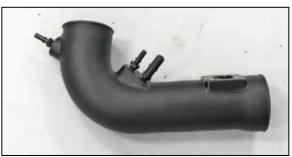
19. Install the quick disconnect fittings into the  $K\&N^{\odot}$  intake tube as shown.
