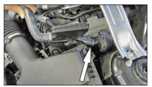
6. Cut the clamp that secures the sound tube/ chamber to the sound drum and then disconnect the sound tube/chamber from the sound drum.
