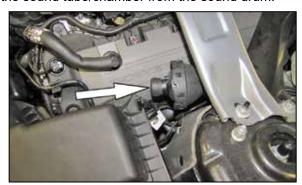
7. Install the provided cap onto the sound drum.
