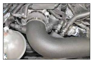
25. Connect the crank case vent, EVAP vent and idle by pass lines to the quick disconnect fittings installed into the K&N® intake tube.
