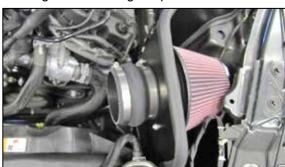
17. Install the provided hump coupler (08418) onto the filter adapter and secure with the provided hose clamp.
