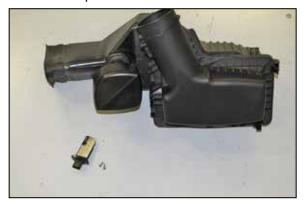
21. Remove the mass air sensor from the factory air filter housing.
