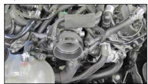
18. Install the provided hump coupler (08699) onto the throttle body and secure with the provided hose clamp.
