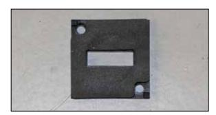
20. Install the provided gasket onto the K&N® mass air sensor adapter.
