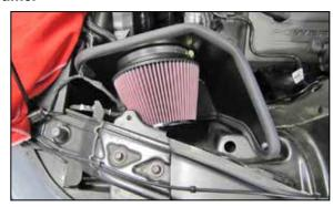
15. Install the K&N® air filter onto the adapter and secure with the provided hose clamp.
