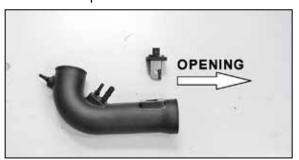
23. Install the mass air sensor assembly into the K&N® intake tube so that the opening in the sensor faces towards the filter end of the tube and secure with the provided hardware.
