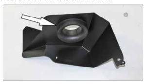
12. Install the provided filter adapter into the heat shield as shown and secure with the provided hardware.
