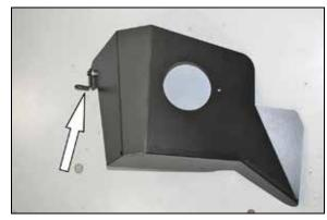
11. Install the provided heat shield mounting bracket (064326) onto the heat shield as shown using the provided hardware.
