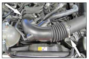
5. Loosen the hose clamps securing the factory intake tube and then remove the intake tube from the vehicle.
