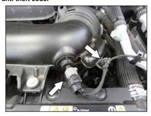
2. Disconnect the inlet air temperature sensor electrical connection and unhook the wiring harness from the intake tube.
