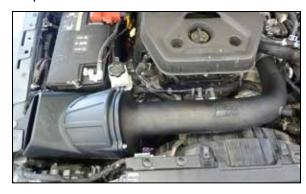
17. Install the intake assembly into the vehicle so the mounting studs insert into the mounting grommets and the intake tube inserts into the coupler. Secure the system with the provided hose clamp and hardware.
