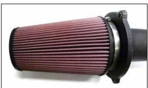
14. Install the air filter onto the end of the K&N<sup>®</sup> intake tube and secure with the provided hose clamp.
