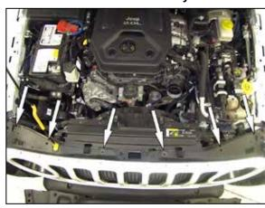
6. Remove the six retaining clips that secure the grill assembly to the core support. Remove the grill assembly.
