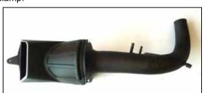
15. Install the intake tube assembly into the K&N<sup>®</sup> air filter housing and secure with the provided hardware.
