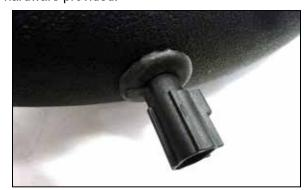
13. Remove the inlet air temperature sensor from the factory intake tube. Remove the O-ring from the sensor and then install the sensor into the K&N<sup>®</sup> intake tube using the provided grommet.
