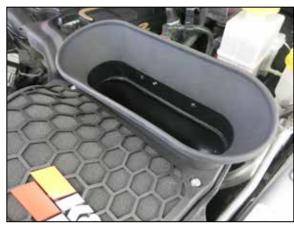
17. Install the fresh air intake seal onto the air filter housing and secure with the provided push pins.
