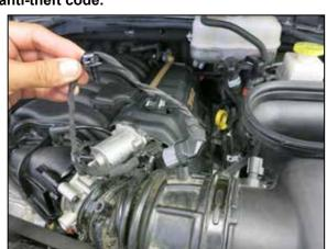
2. Disconnect the IAT sensor electrical connection and unhook the wiring harness from the intake tube.
