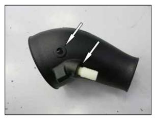
7. Install the provided CCV fitting and IAT grommet into the K&N intake tube as shown.
