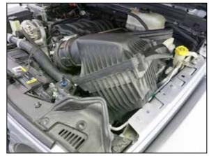
6. Remove the complete air filter housing from the vehicle.
