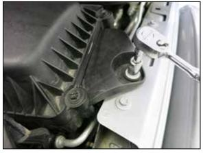
3. Remove the bolt that secures the factory air filter housing to the inner fender.
