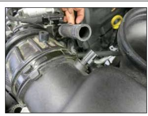
5. Release the spring clamp that secures the CCV hose to the factory air filter housing port and then disconnect the CCV hose from the port.
