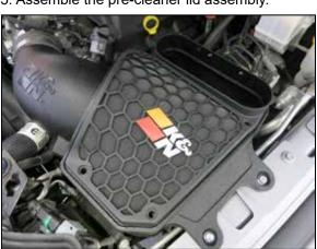
16. Install the pre-cleaner lid assembly onto the K&N filter housing and secure with the provided hardware.
