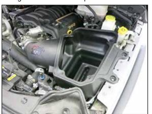
10. Set the K&N intake system into position so the coupler engages the throttle body and the posts on the bottom of the filter housing engage the factory mounting grommets. Secure the filter housing to the inner fender with the provided hardware. Secure the coupler to the throttle body with the provided hose clamp.
