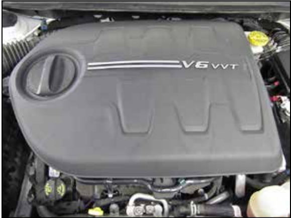
2. Lift off the engine cover and set aside.
