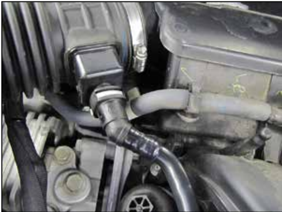
3. Release the locking tab and disconnect the crank case vent line from the factory intake tube.
